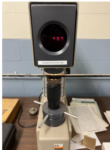
Figure 4.9 Rockwell C Hardness Test Apparatus.
