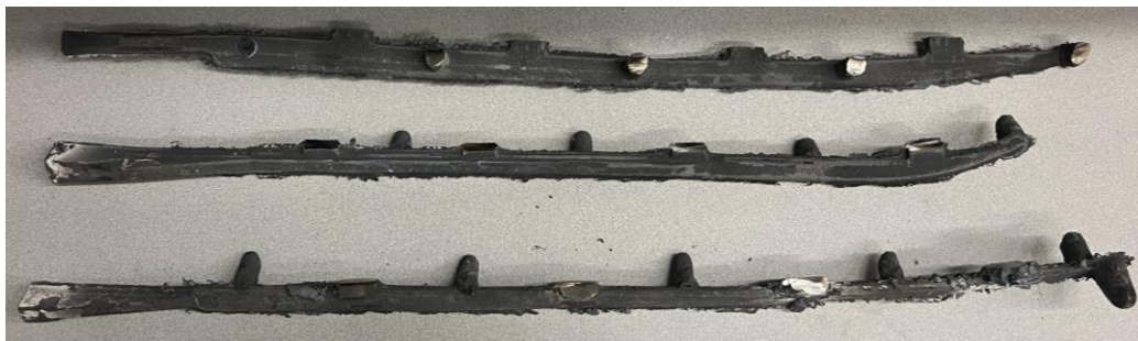
Figure 4.5 Casting Results of Pour 3. Blades 6, 3, and 7 From Top to Bottom.
