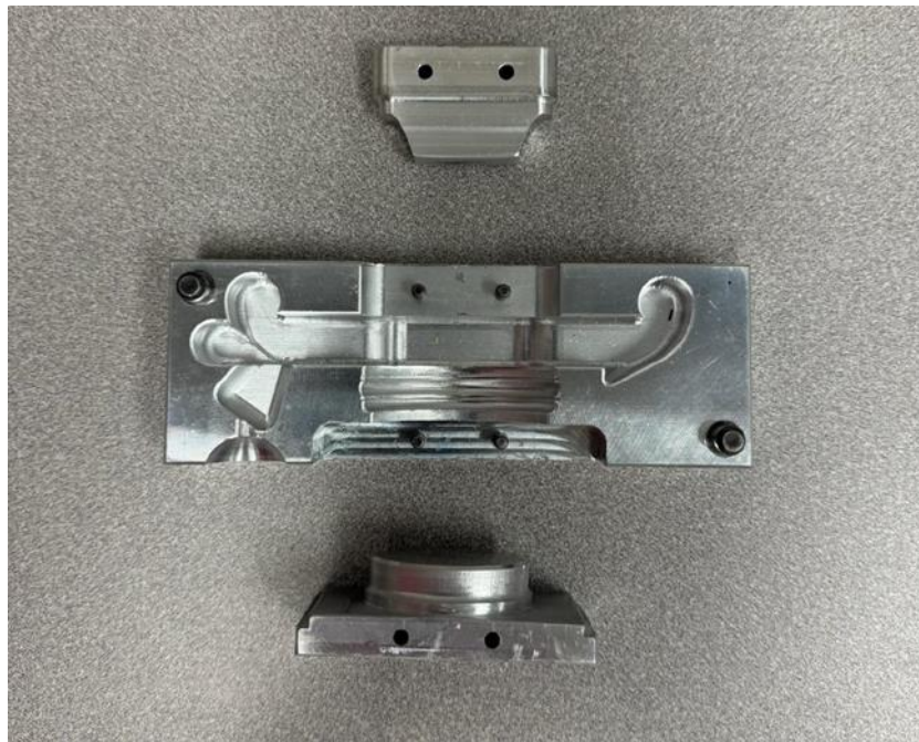
Figure 5.1: A wax injection die designed with cores to produce wax patterns of Casting A.
