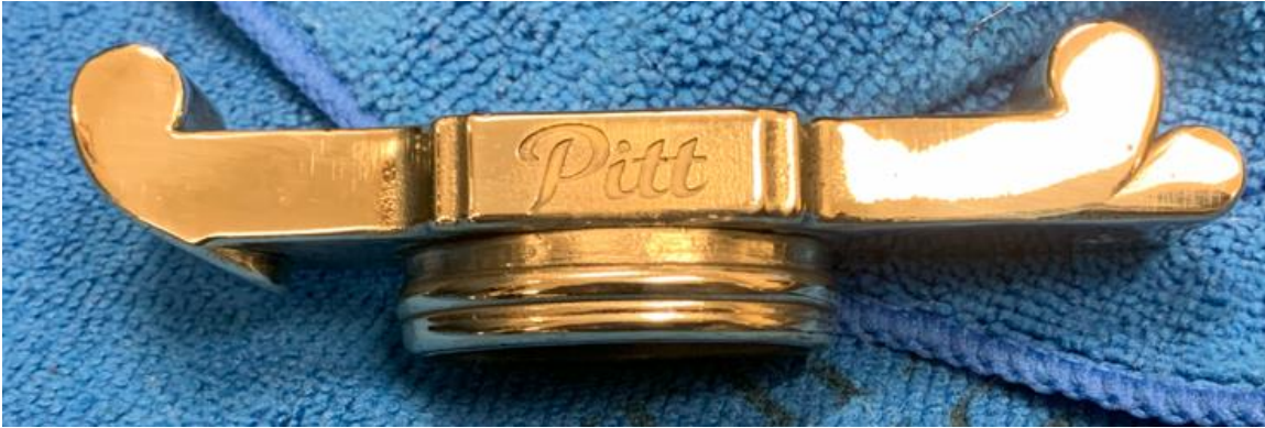
Figure 6.3: Casting B fixture for the floral engraving operation on the knucklebow.
