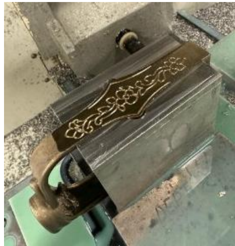
Figure 6.4: Casting B fixture for the SFSA engraving operation on the pommel.
