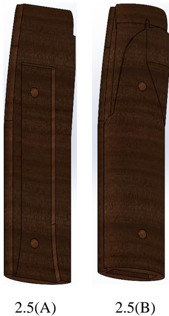
Figure 2.5: A & B images depicting the handle of the sword, which was derived using the cavity function within SolidWorks.
