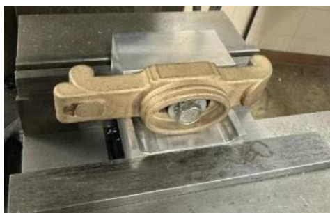
Figure 5.3: Casting A fixture for the “Pitt” engraving operation.
