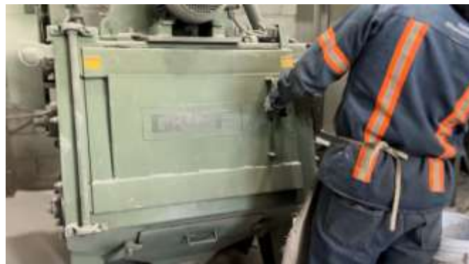
Figure 7.2 Shot Blasting Process on Pommel and Guard
