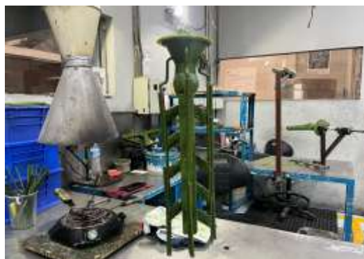
Figure 5.4.1 Vertically Designed Wax Tree for Casting
