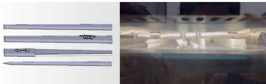
Figure 5.1. 3D printing of the sword blade in 4 parts
