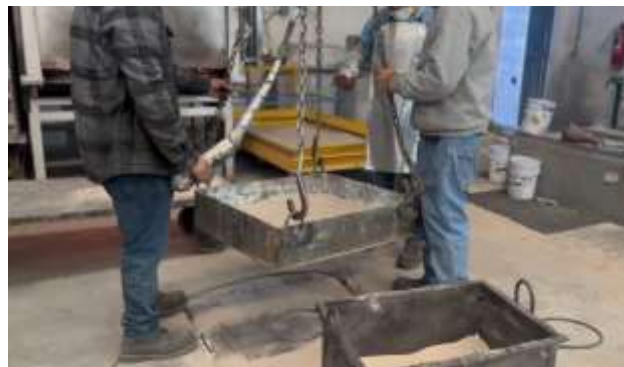
Figure 5.7.1. Mold Secured on Metal Support Before Pouring
