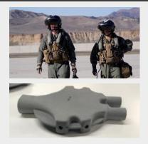
Four suppliers produced these manifolds components from glass-reinforced nylon
