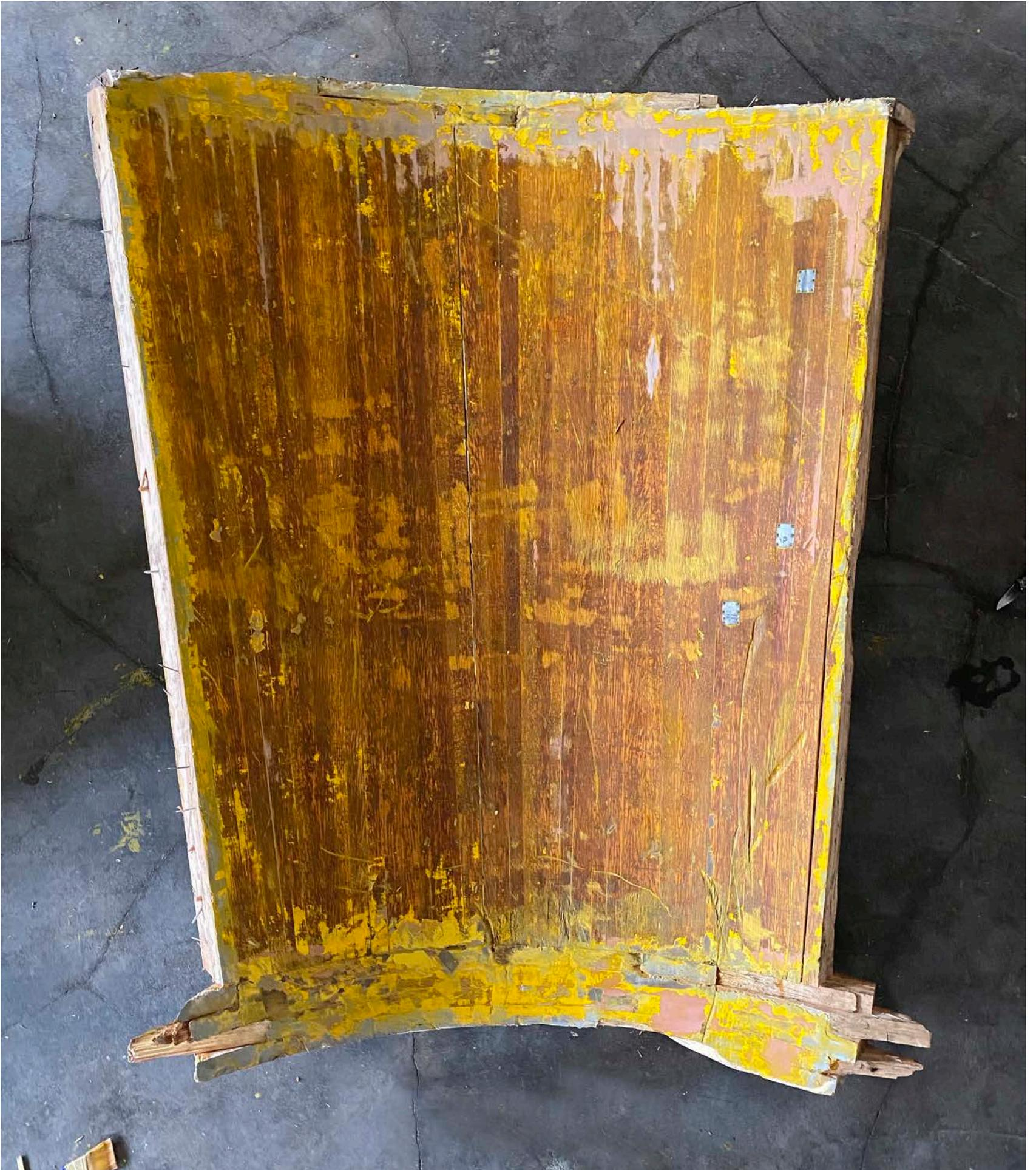
Cleaned and stripped Wooden casting mold salvaged from WHEMCO, preparation for painting.
