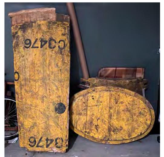
Rough wooden casting mold fragments before cleaning and preparation for painting.
