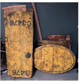
Rough wooden casting mold fragments before cleaning and preparation for painting.
