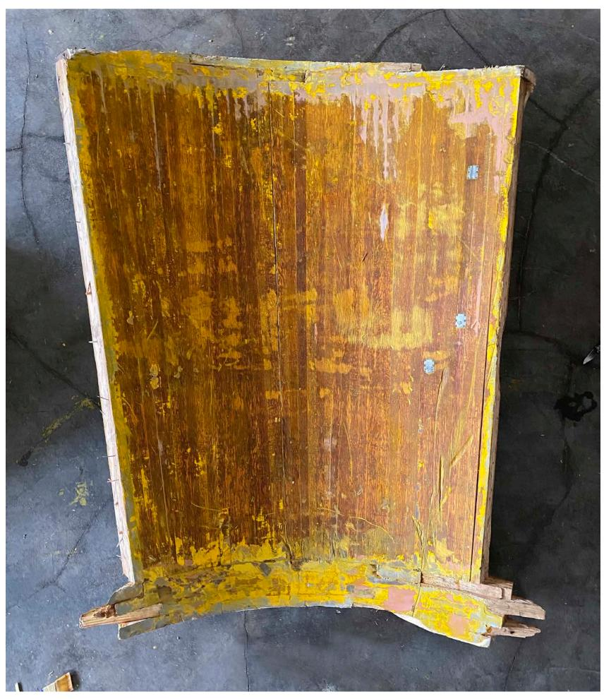
Cleaned and stripped Wooden casting mold salvaged from WHEMCO, preparation for painting.
