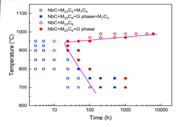
TTT diagram of HP40NB alloy determined from X-ray diffraction data by *Fuyang et. al.*<sup>2</sup>
