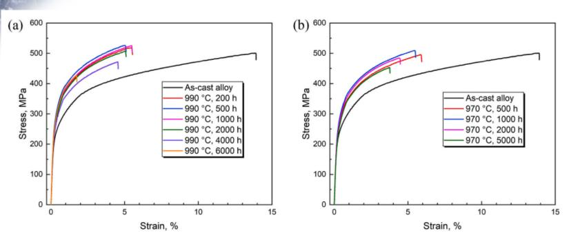
Tensile stress strain plots of HP40NB alloy after aging at (a) 990°C and (b) 970°C from Fuyang et. al. 1
