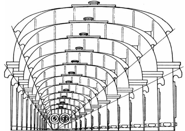
Figure 1. Display of a gearbox size range (Koller 1998, p. 328).
