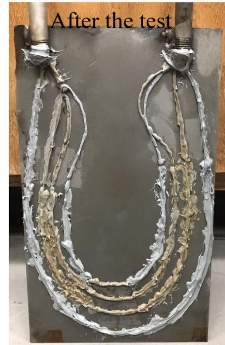
Heating the plate in a box furnace at 200 °C for ~2 hours and then spraying water in a quench tank at 50-65 psi for ~4.5 hours
