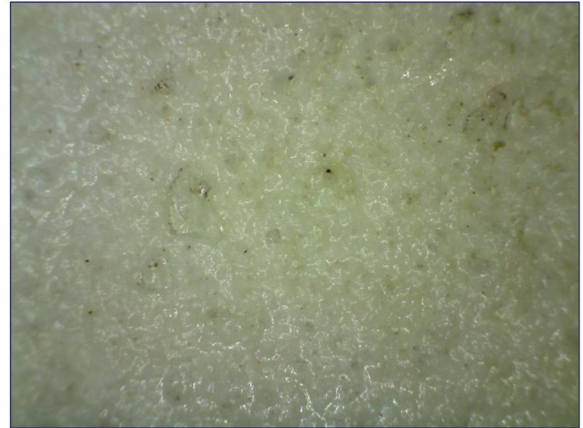
Sintered at 1280C
