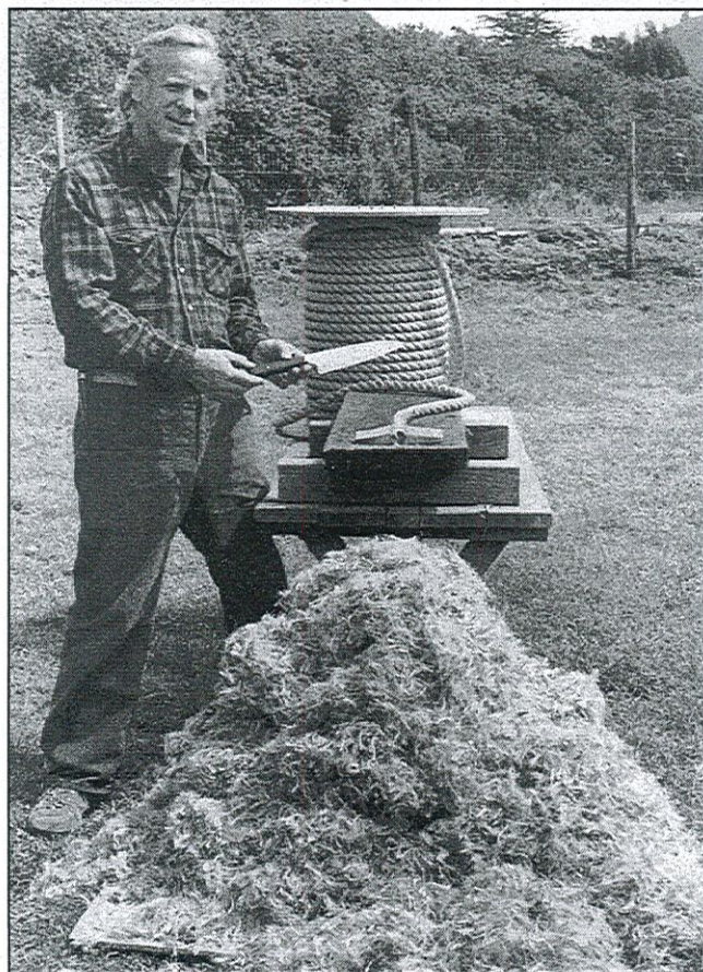
This pile of hemp particles is the result of fifteen hours used to make 3000 cuts in 1-inch rope, using an 8-inch Boye dendritic steel knife. This was done without resharping the blade.
