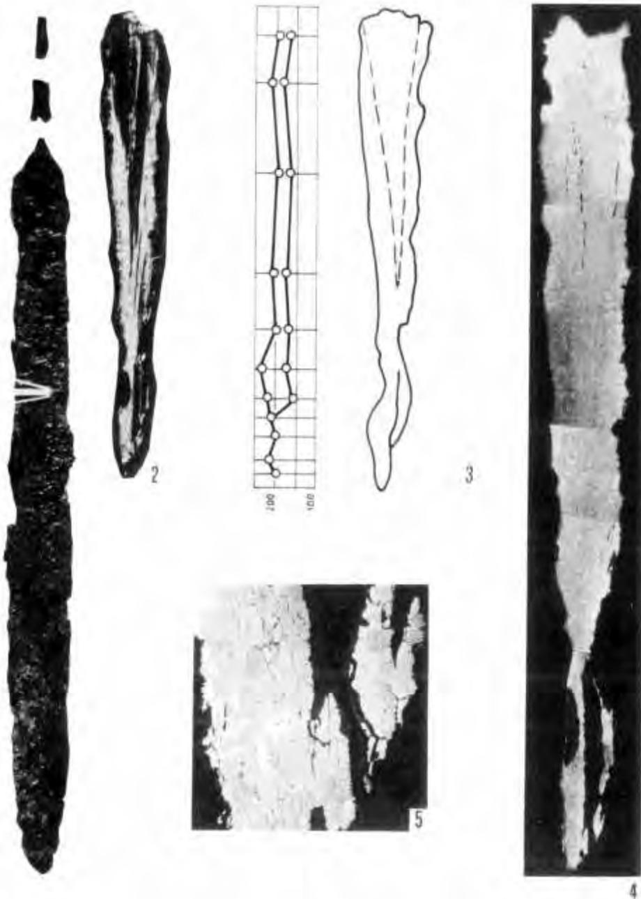
IV. Makotřasy 587, central Bohemia, examination 6. 1 Blade, with specimen position marked; 2 Cross-section, etched with Oberhoffer: a wedged shaped core with elevated phosphorus content ( $\times 7$ ); 3 Microhardness 30 g, and a cross-section sketch, showing principal inclusion chains; 4 Cross-section composed from microphotographs, ferrite, etched with 2%-Nital ( $\times 15$ ); 5 Cutting-edge: deformed ferrite grains ( $\times 100$ ), etched with 2%-Nital
