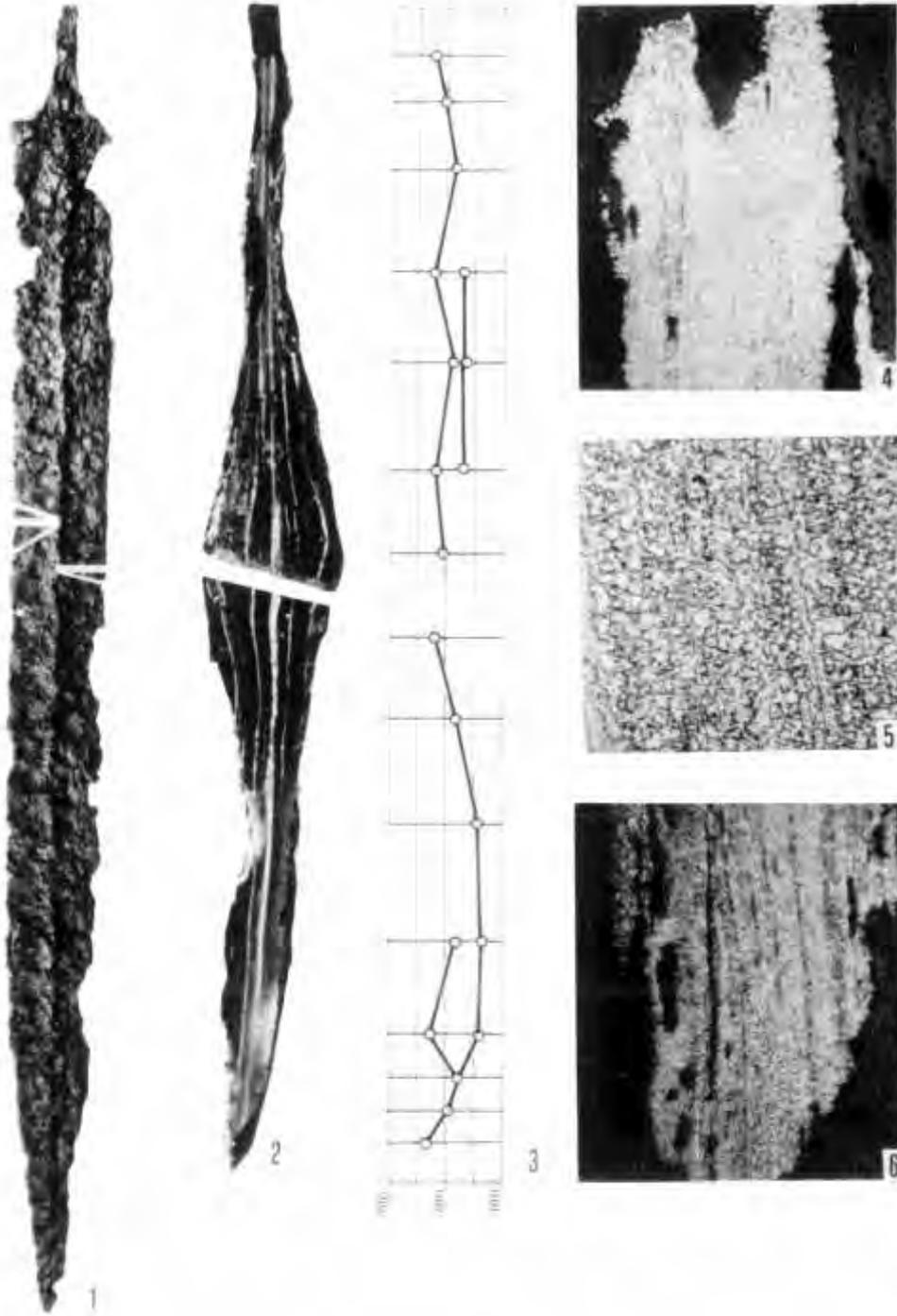
XXI. Holubice 599, examination 17. 1 Blade, with specimen positions marked ( $a_1$  left,  $a_2$  right); 2 Composite cross-section, etched with Oberhoffer (laminated texture,  $\times 5$ ); 3 Microhardness 30 g; 4 Cutting-edge  $a_2$  ( $\times 100$ ); 5 The same specimen, far from edge, ferrite ( $\times 150$ ); 6 Cutting-edge  $a_1$ : ferrite with traces of pearlite ( $\times 75$ ). 4–6 etched with 2%-Nital
