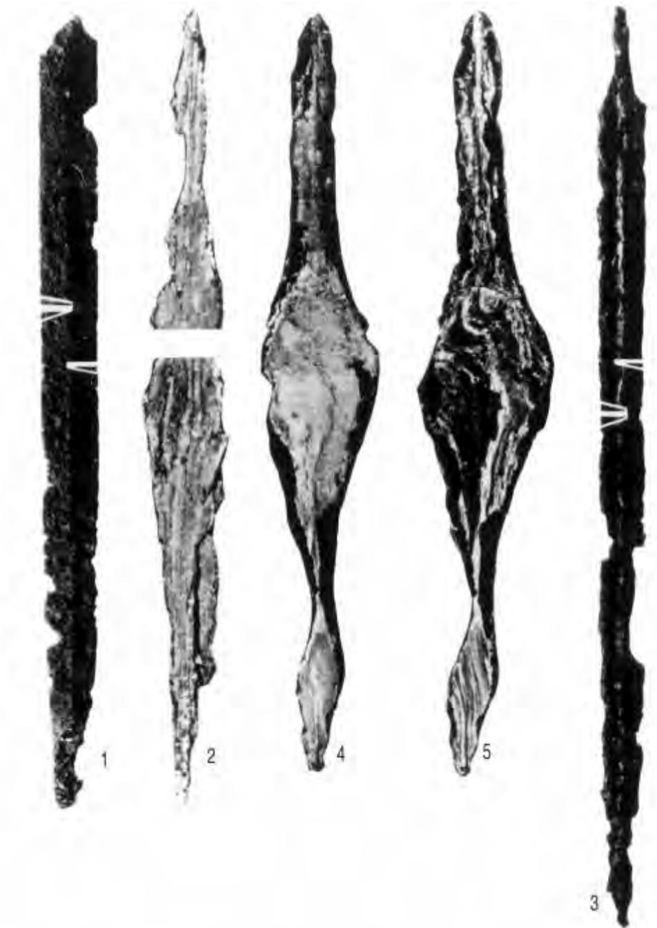
XIV. Brno-Maloměřice 593 and 594, examinations 11 and 12. 1 593 with specimens positions marked ( $a_1$  left,  $a_2$  right); 2 593; composite cross-section, showing lamination, etched with Heyn ( $a_1$  above,  $\times 8$ ); 3 594: cross-section composed from  $a_1$  (lower cutting-edge) and  $a_2$ , and etched with Heyn ( $\times 6$ ); 4 The same, etched with Oberhoffer: distorted bands with varying phosphorus content; 5 594: with specimen positions marked ( $a_1$  left,  $a_2$  right)
