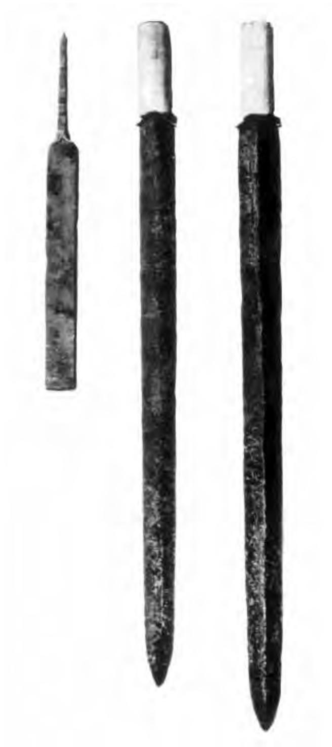
I. Experimental forging of La Tène type sword-blades. *Left:* Bar of the 'saumon d'épée' type (after an original in Landesmuseum Zürich, found at Port, Switzerland), *Centre:* Sword *A* with flat blade (lenticular cross-section). *Right:* Sword *B* with central rib (lozenge-shaped cross-section). The hilts shown are not intended as reconstructions
