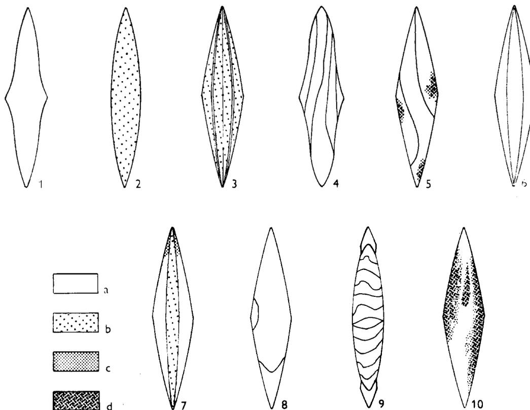
Fig. 14. Selected examples of wrought-iron or mild steel blade-constructions.
