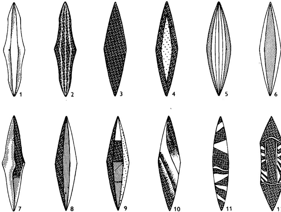
Fig. 17. Reconstructions of important blade-constructions (hardenable steel over 0.3 per cent C)
