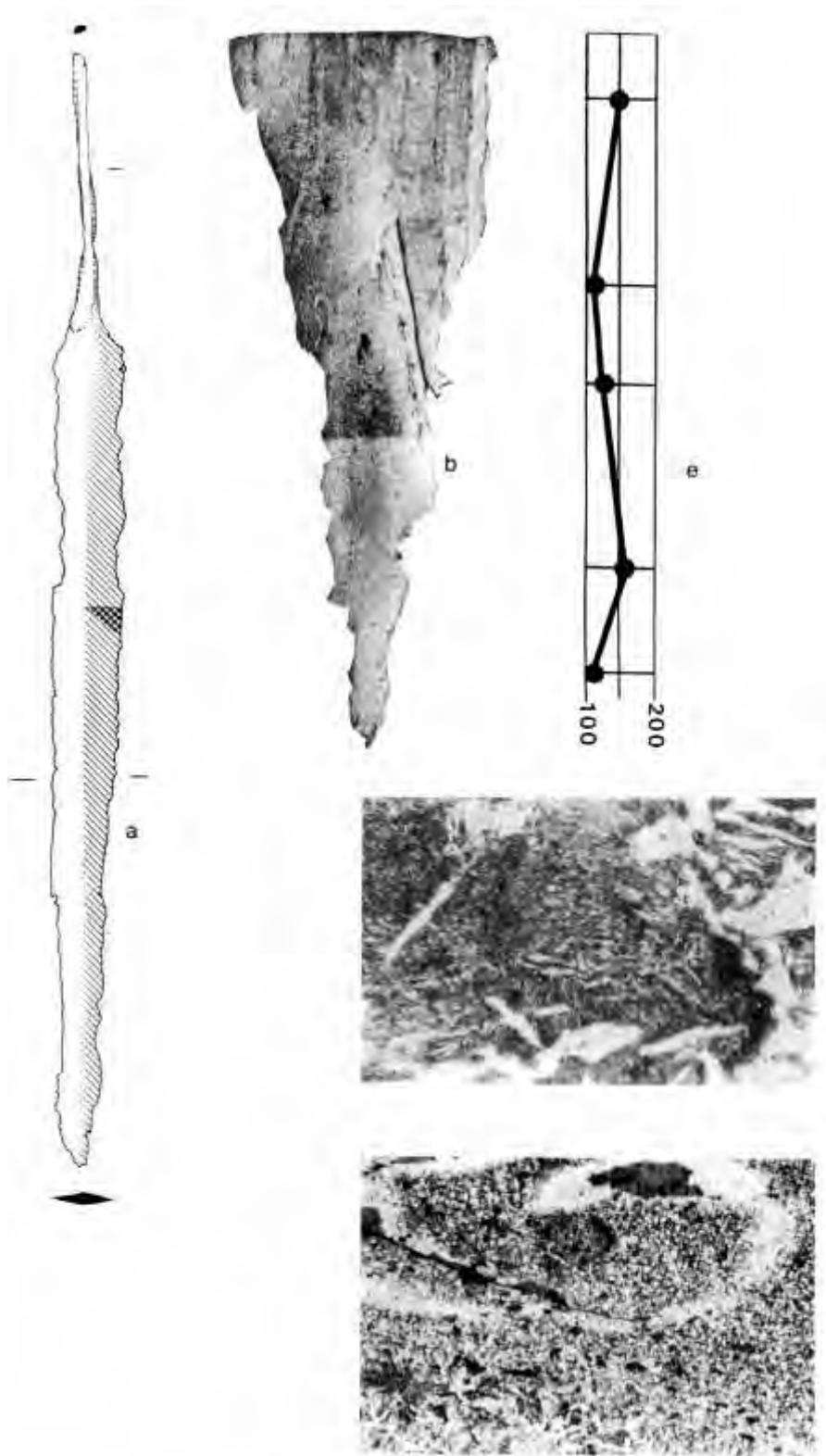
XXXVI. Kildrinagh 1, Ireland, examination 91. (a) Sword  $\times 2/5$ ; (b) Macrostructure; (c) Pearlite showing spheroidization of carbides  $\times 500$ ; (d) Remains of bloom welds  $\times 50$ ; (e) HV profile. Etched 4%-Nital. (After Scott 1990.)
