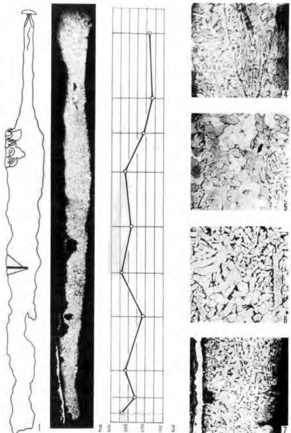
XI. Třebohostice 178, S. Bohemia, examination 8. 1 Blade with specimen position marked; 2 Transversal section, composed from microphotographs,  $\times 23$ ; 3 Microhardness 30 g; 4-5 Ferritic structures with intergranular pearlite in various parts of the section; 6 a wedge-shaped weld; 7 Adherent thin layer of a copper-based metal (on left). Etched with 2%-Nital. Magnifications: 4 and 7 ( $\times 100$ ); 5 and 6 ( $\times 150$ )
