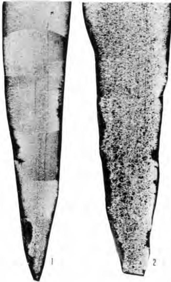
XXXI. Zemplín 510. 1 Specimen *a*, composed from microphotographs ( $\times 20$ ): ferritic-and-pearlitic steel, weld-seams; 2 Specimen *b*: pearlitic structure (dark) with ferritic cells and needles ( $\times 30$ ).
