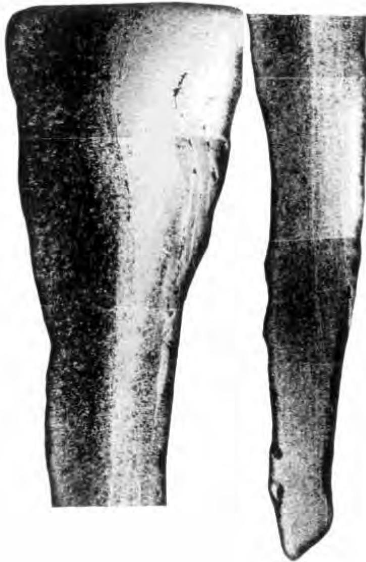
XXIX. Holubice 606, cutting-edge  $a_2$ , composed from microphotographs: a pearlitic steel band (dark), joint with wrought iron by welding ( $\times 26$ ). Etched with 2%-Nital
