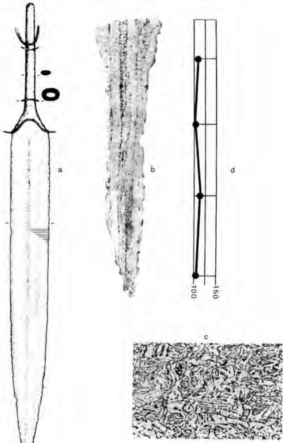
XXXV. Lisnacrogher 3, Ireland, examination 90. (a) Sword  $\times 2/5$ ; (b) Macrostructure; (c) Elongated ferrite grains with interstitial perlite  $\times 100$ ; (d) HV profile. Etched 4%-Nital. (After Scott 1990.)
