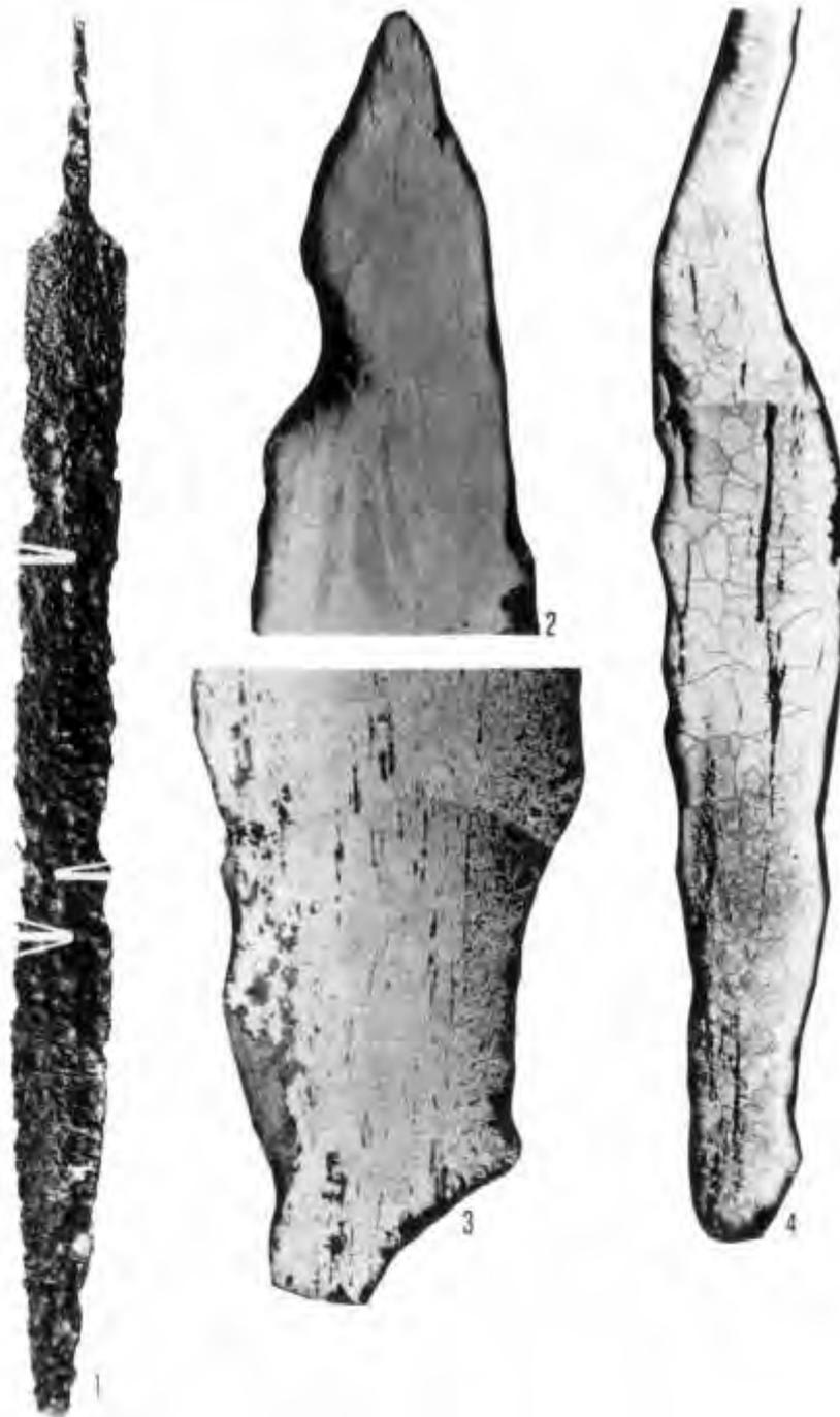
XXIV. Holubice 602, examination 20. 1 Blade, with specimen positions marked ( $a_2$  right,  $a_1$  left, and  $b$  above it); 2 Cutting-edge  $a_2$ : coarse ferrite, deformed ( $\times 100$ ); 3 Cutting-edge  $a_1$ : ferrite, at right a surface layer of pearlitic-and-ferritic network and needles, numerous dark slag inclusions, ( $\times 100$ ); 4 Cutting-edge at  $b$ : ferrite with varying grain size ( $\times 100$ ). Etched with 2%-Nital
