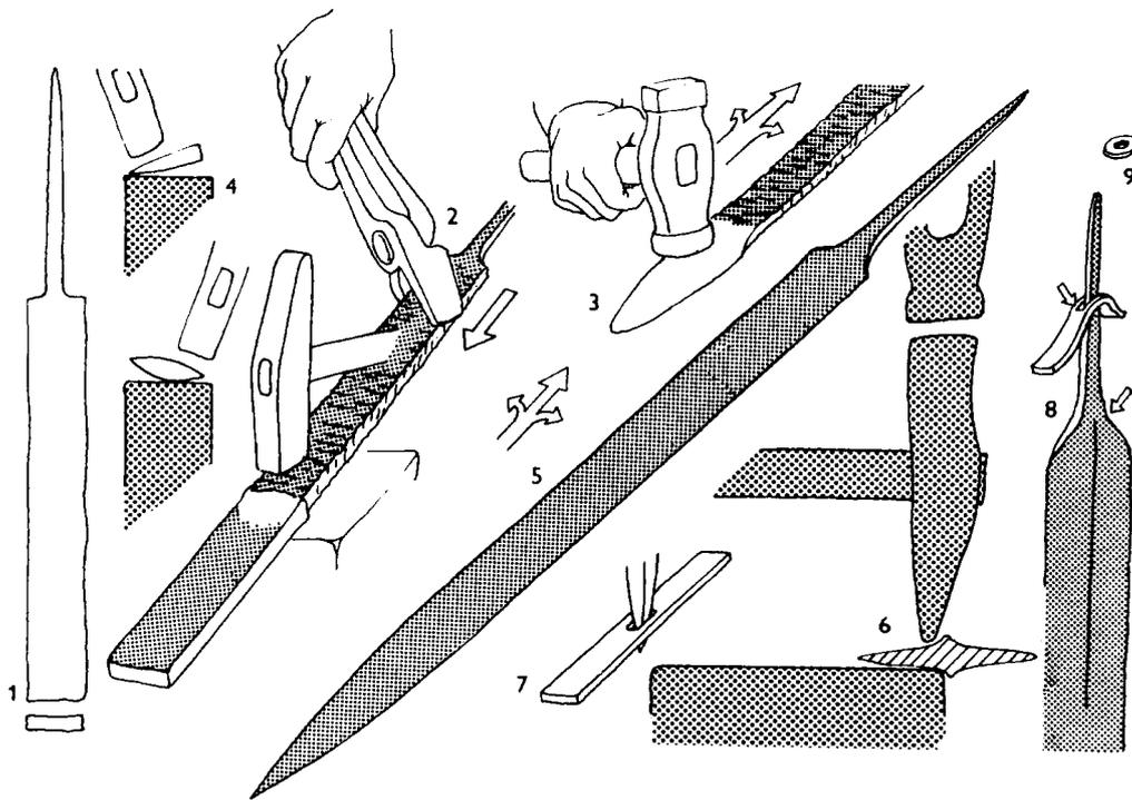
Fig. 8. Experimental forging of La Tène type sword-blades (1982)
