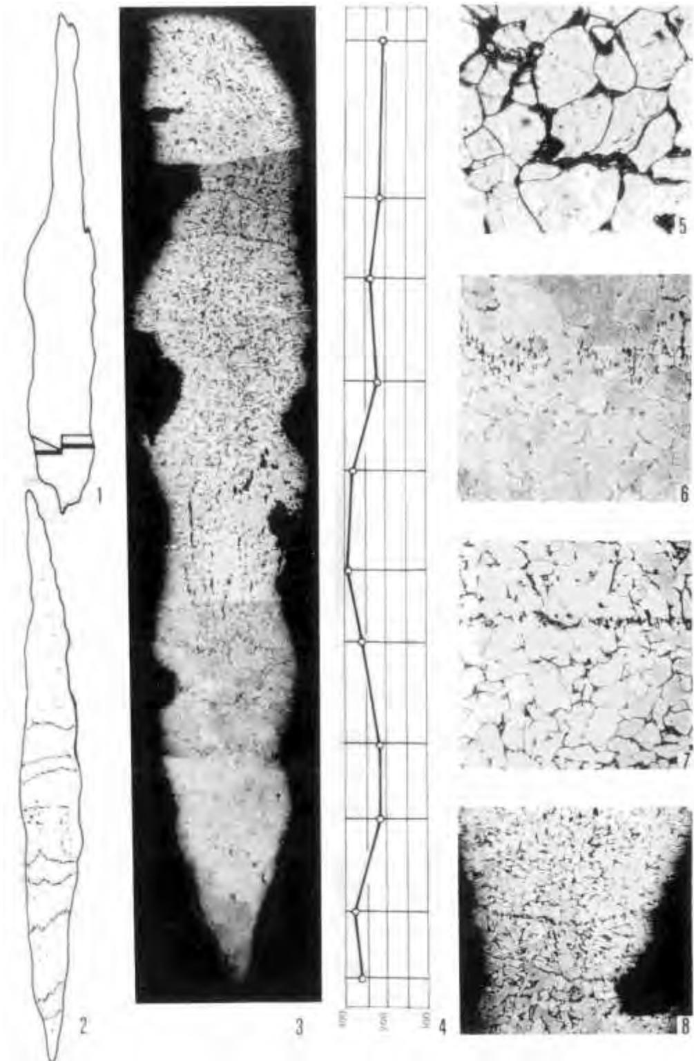
XII. Třebostice, 179, examination 9. 1 Blade with cross-section marked; 2 Schematic sketch of the cross-section, composed from parts *a* and *b*; transverse welds; 3 Cross-section part *a*, composed from microphotographs, ( $\times 4$ ); 4 Microhardness 30g; 5 Ferrite with intergranular pearlite ( $\times 250$ ); 6–8 Similar structures with transversal welding-seams, (6–7  $\times 100$ ; 8  $\times 75$ ) Etched with 2%-Nital
