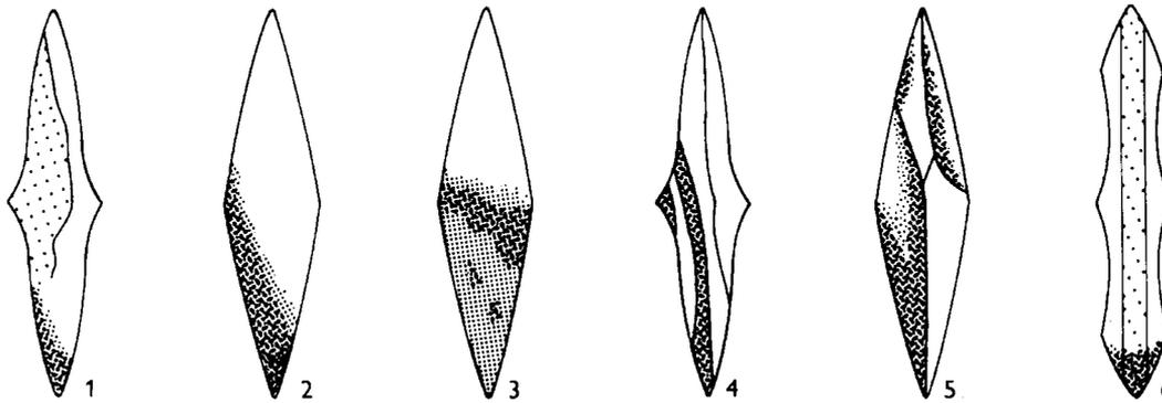
Fig. 18. Interpretation of some one-sided blade-constructions (with steel in one cutting-edge only)
