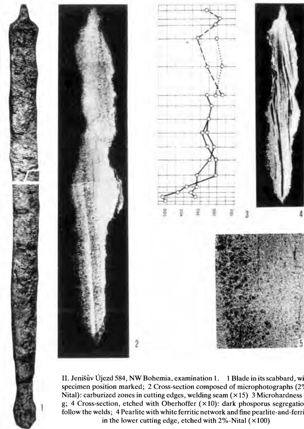
II. Jenišův Újezd 584, NW Bohemia, examination 1. 1 Blade in its scabbard, with specimen position marked; 2 Cross-section composed of microphotographs (2%-Nital): carburized zones in cutting edges, welding seam ( $\times 15$ ) 3 Microhardness 30 g; 4 Cross-section, etched with Oberhoffer ( $\times 10$ ): dark phosphorus segregations follow the welds; 5 Pearlite with white ferritic network and fine pearlite-and-ferrite in the lower cutting edge, etched with 2%-Nital ( $\times 100$ )
