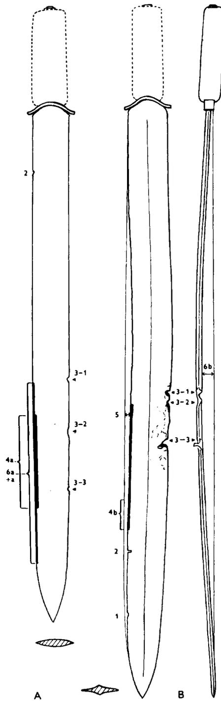
Fig. 20. Deformation of the test blades caused by experimental strokes
