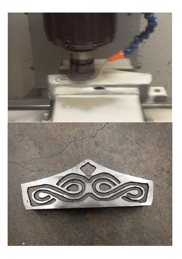
Following machining, the hammer went through heat treating to increase its hardness. To heat treat, we held the hammer head in a furnace for 2 hours a 700° C, followed by quenching in oil. After the hammer was cool enough to remove from the oil, it was left to air cool. Heat treating and quenching also gave the hammer a dark appearance and highlighted the runic design more, finishing the appearance of the head itself.
