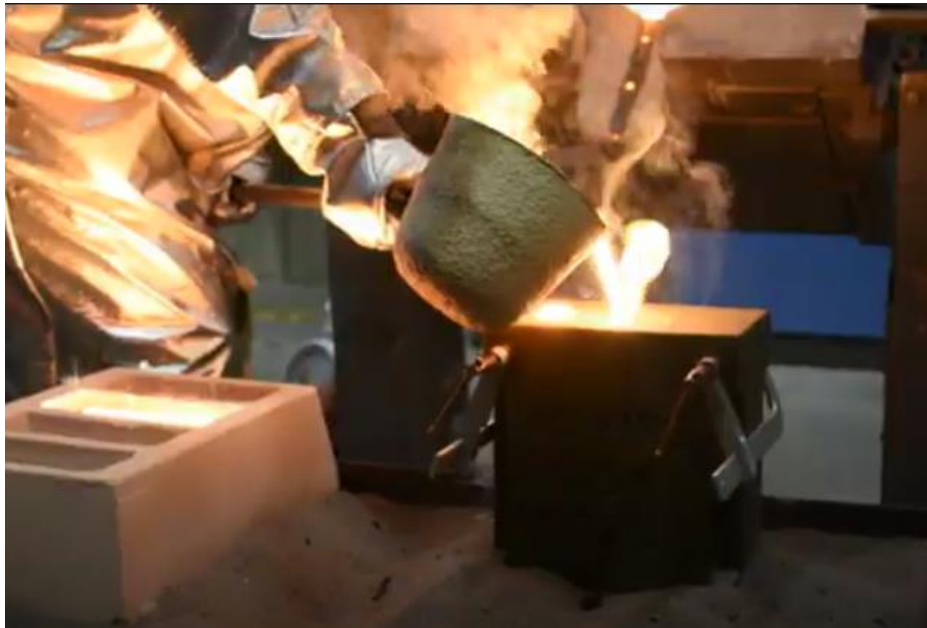
Figure 13. The hand ladle had two grams of aluminum added before it was used to hand pour the mold.
