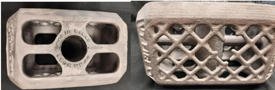
Figure 24. The lettering and cores did not shift, but the lattice still did not fill completely.
