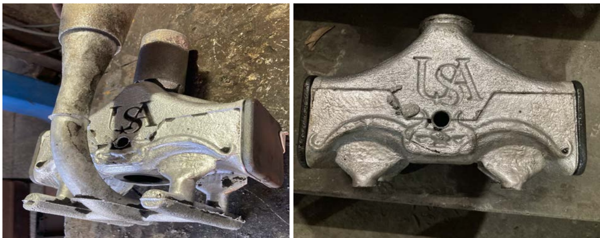
Figure 22: The composite part with its gates and risers (left) and after they were removed (right).
