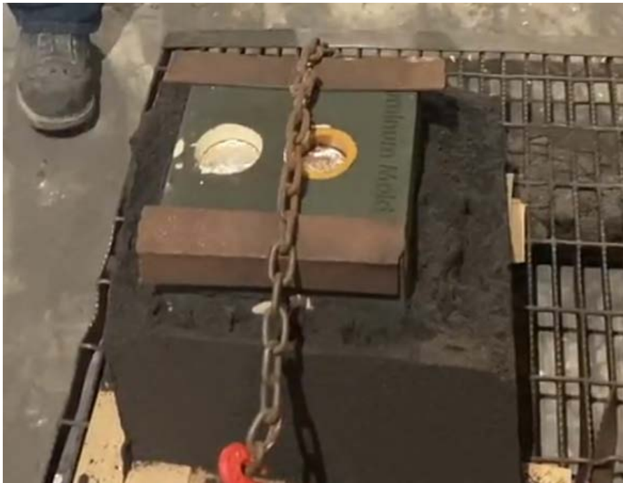
Figure 20: The assembled aluminum casing mold (green block in the middle) and the exterior block (black block surrounding it).
