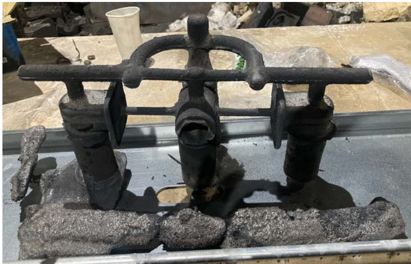
Figure 21: The steel core with the gates and risers after being removed from the mold.
