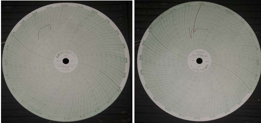
Figure 23: Logs of the two heat treatments done on the steel core before the aluminum casting.
