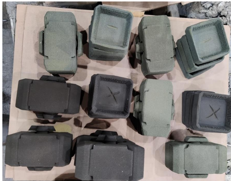
Figure 11 - Balance of the cores and inserts. Green parts are Silica, brown parts are carboceramic.
