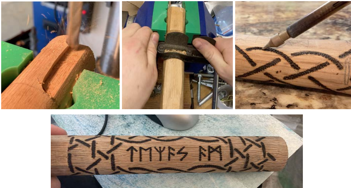
Figure 7. Steps to create the handle, including milling, shaping, wood burning, and the final part
