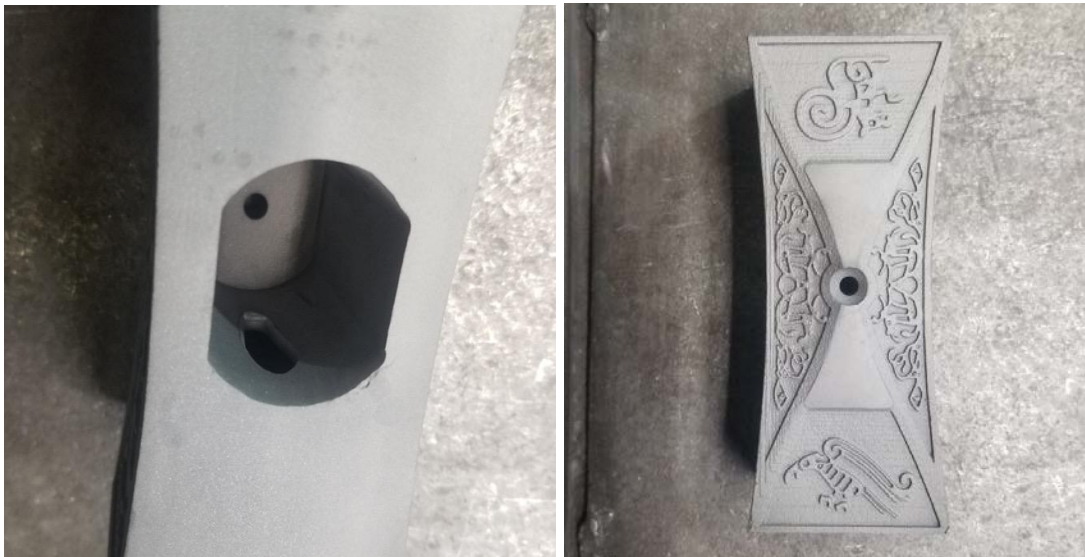
Figure 11. Pictures of the bottom with emergency epoxy fill-holes and the top with the gates.
