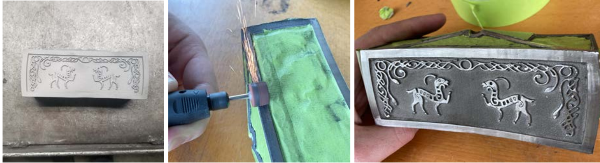
Figure 8. Pictures of the hammer head before, during, and after polishing
