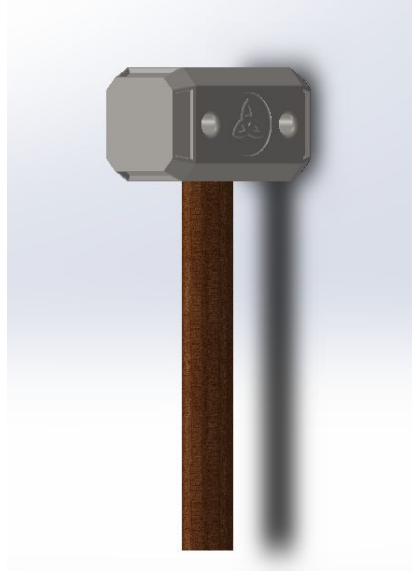
Figure 7. An isometric view of a section of the weight reduced scale hammer. Dimensions: 2.49" by 4.3" by 10.0"
