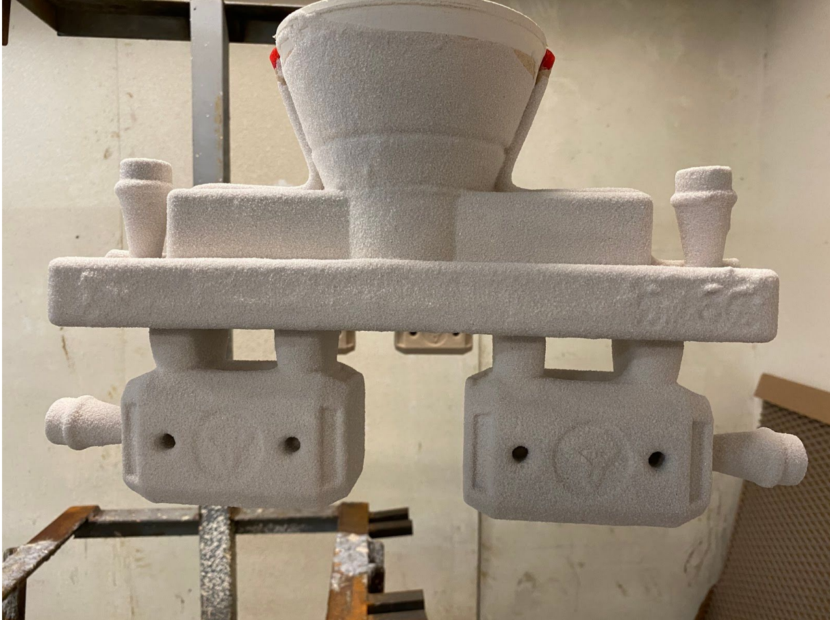
Figure 9. A picture of the final casting tree with two hammer heads, venting system, and casting gates.
