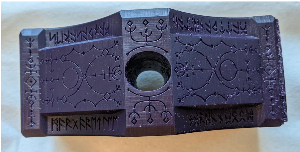
Figure 4 This is our 3D wax printed hammer.
