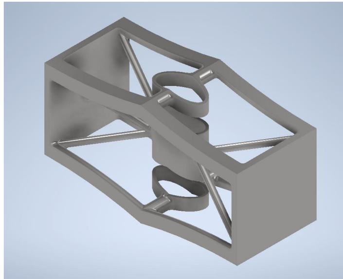
*Figure 3; Internal Design of Hammer*
