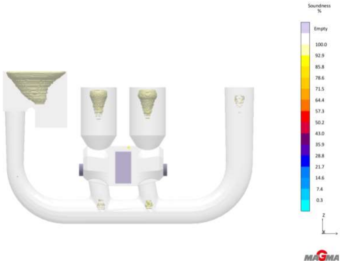
Figure 6: MAGMASOFT simulation rendering of the general soundness of the casting and gating system with a unified scale gradient
