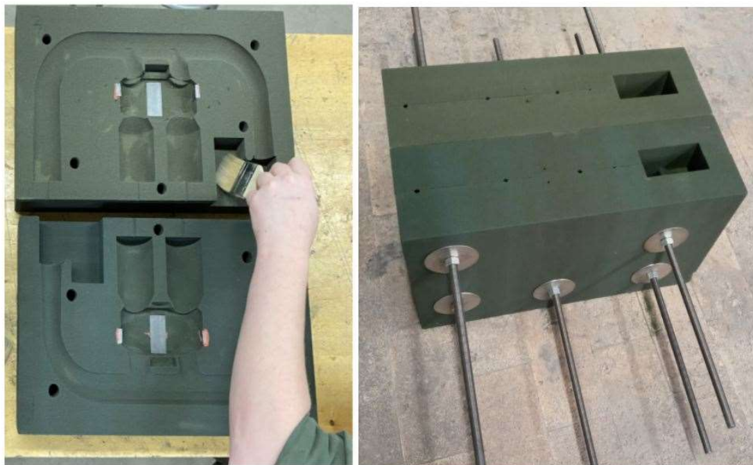
Figure 16: 3D printed sand molds being prepped for a steel pour Sara Roman brush cleaning and a pair of closed molds
