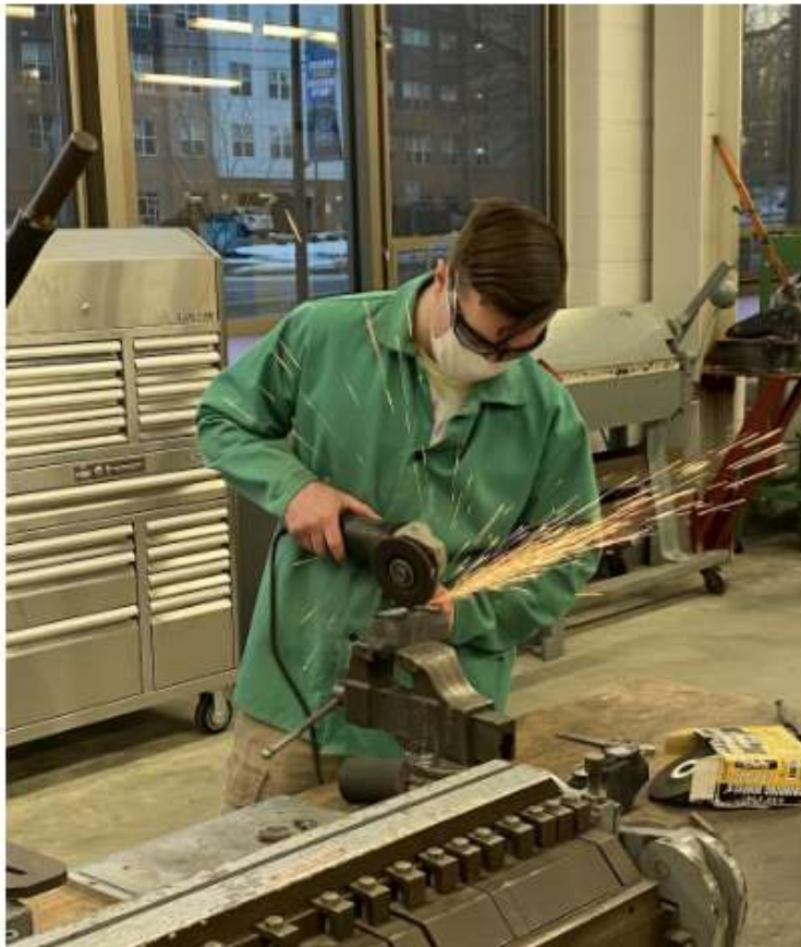
Figure 20: Dan Yost cleaning casting surface with an angle grinder
