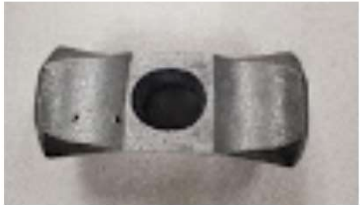
Figure 18: Under riser porosity revealed after the Pentair shot blast
