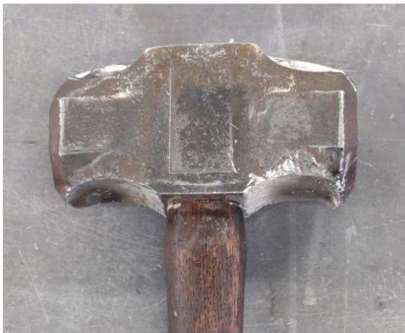
Figure 19: Before shot peening on test handle
