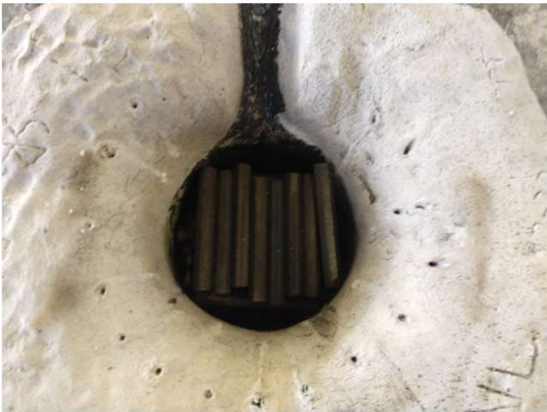
Figure 15: Top down view of the Ajax Tocco 100 pound capacity furnace charged with 60 pounds of 9260 bar stock cut to length and stacked in a Lincoln log style tower
