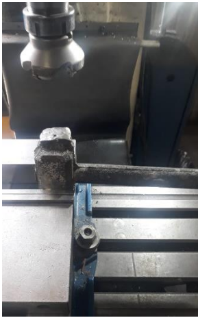
Figure 13. Hammer after being cut and cleaned.
