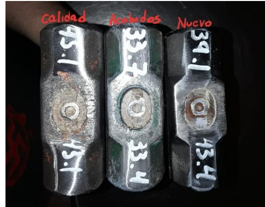
Figure 26. Conventional Hammers with measurements values on them in HRC.
