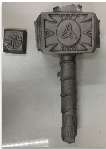
Figure 19. Hammer and the window separated after the arc air and Sandblast process.
