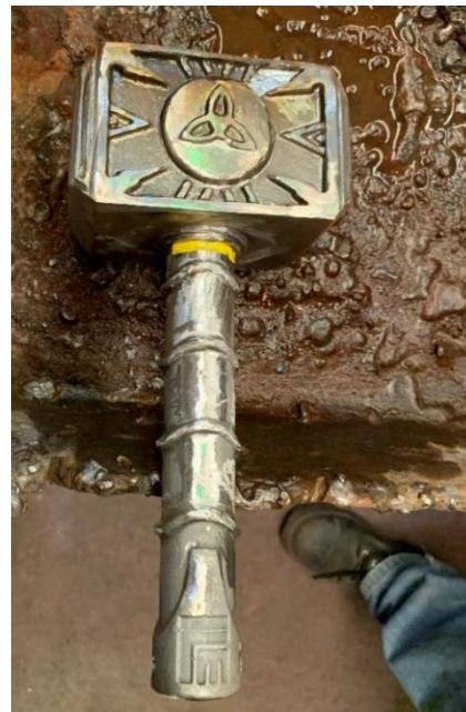
Figure 31. The yellow line indicates the position of the possible crack.
