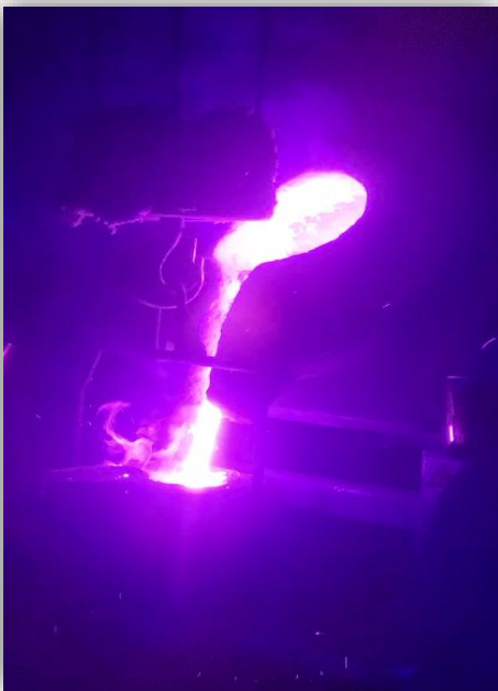
Figure 17. Casting from Induction furnace to Ladle furnace using blue cobalt filter.
