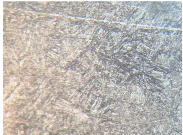
Figure 30. CA6NM alloy, normalized 2h in furnace cooling at 1050°C (1922°F) and tempered 1h in air cooling at 580°C (1076°F). Structure consists of tempered Martensite Virella's reagent 400X
