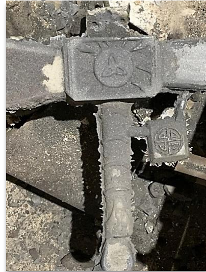
Figure 18. Thor's hammer after an hour of being poured.
