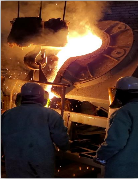
Figure 16. Casting from Induction furnace to Ladle furnace
