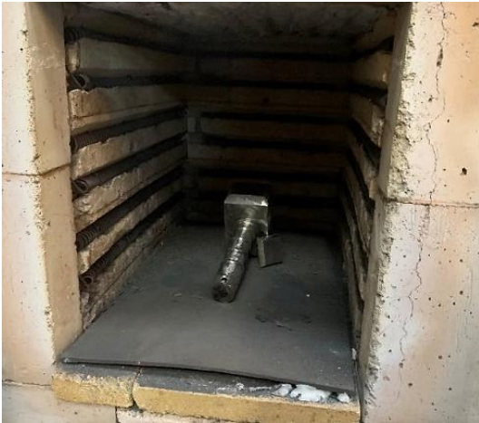
Figure 25. Tempering at 580°C (1076°F) sample No.1.
