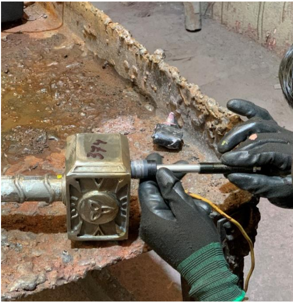
Figure 32. Taking hardness on Thor's hammer.
