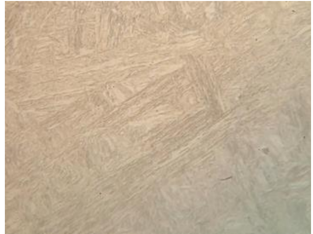
Figure 29. CA6NM alloy, normalized 2h in furnace cooling at 1050°C (1922°F) Structure consists of Martensite, Virella's reagent 400X
