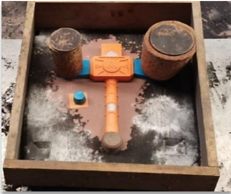
Figure 10. Start of de molding process.
