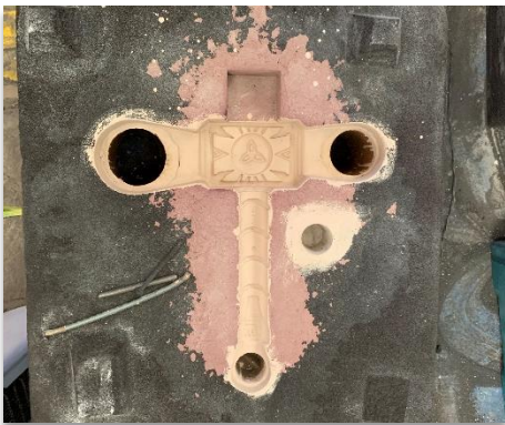
Figure 11. Half-mold in the final stage, with wash coat.
