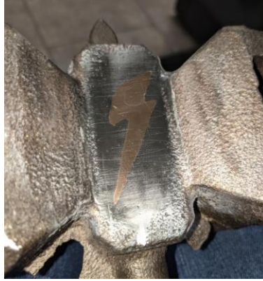
Figure 13. Brass piece integrated into the lightning bolt to provide color contrast
