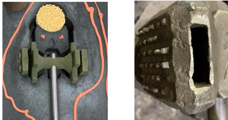
Figure 12. Titanium rod placed in a mold (left) and misruns present on hammer due to chilling during first run (right)
