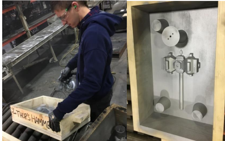
Figure 10. Spraying mold release agent on the tooling
