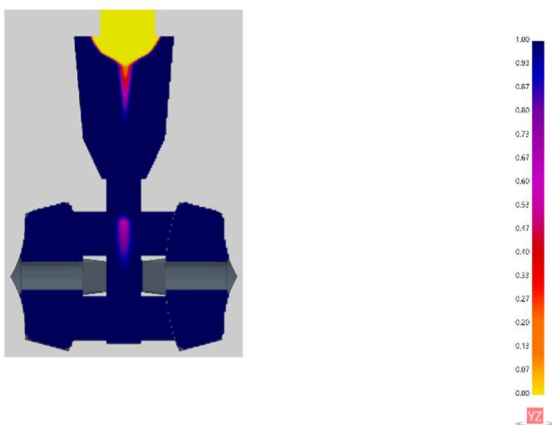
Figure 35: Final Gating Design Density
