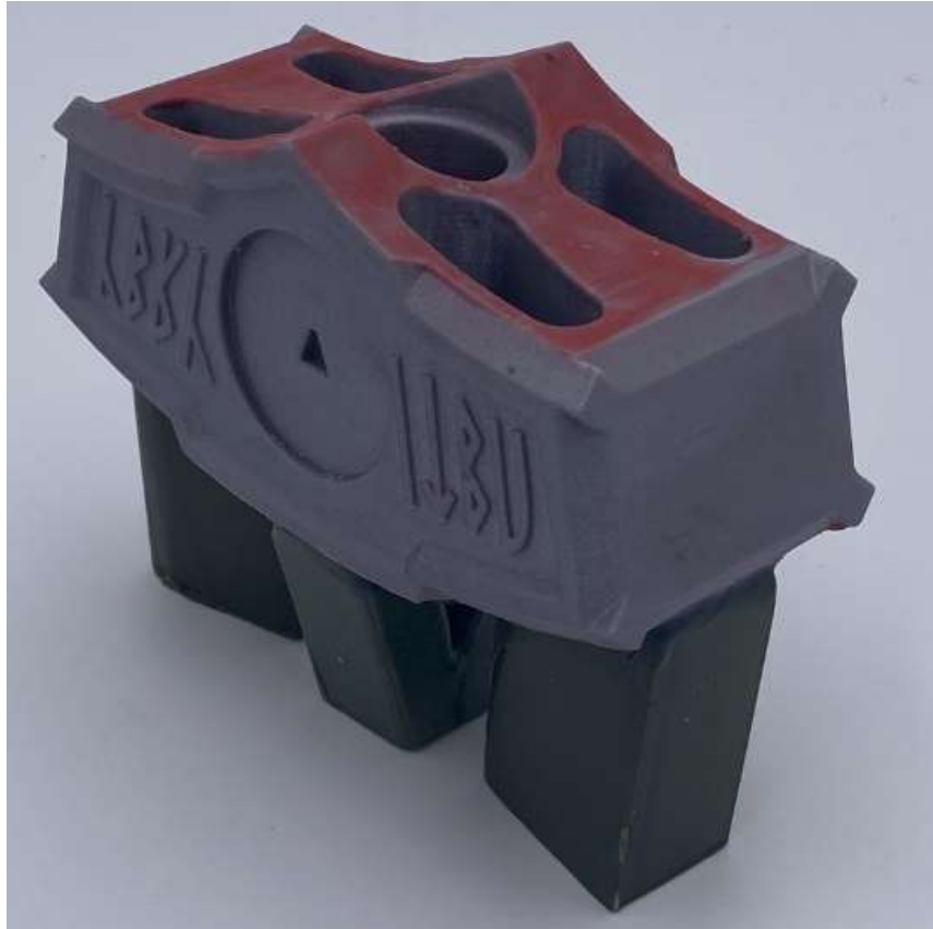
Figure 23: Pattern with Wax Gating
