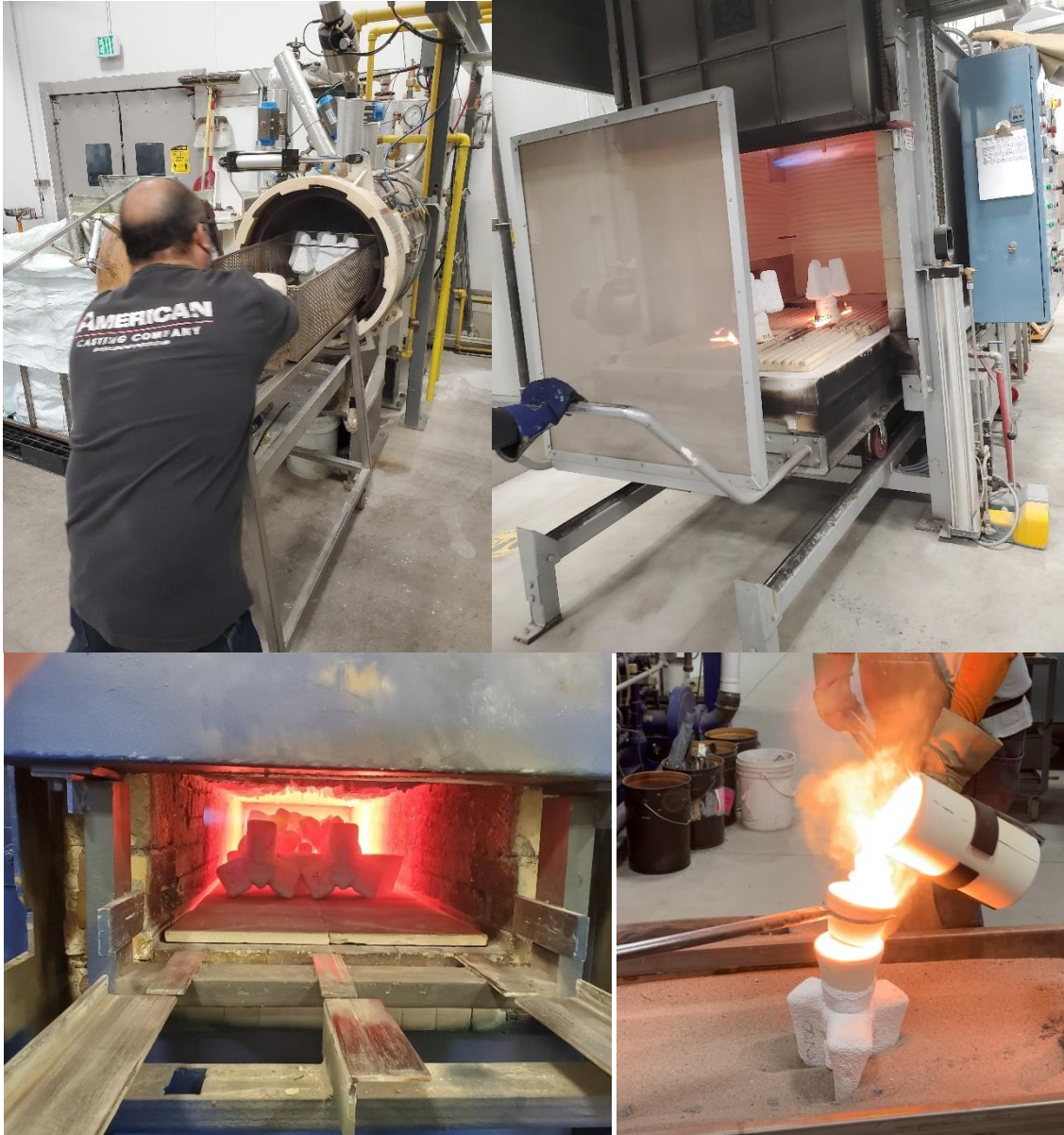
Figure 9 Investment Casting Process
