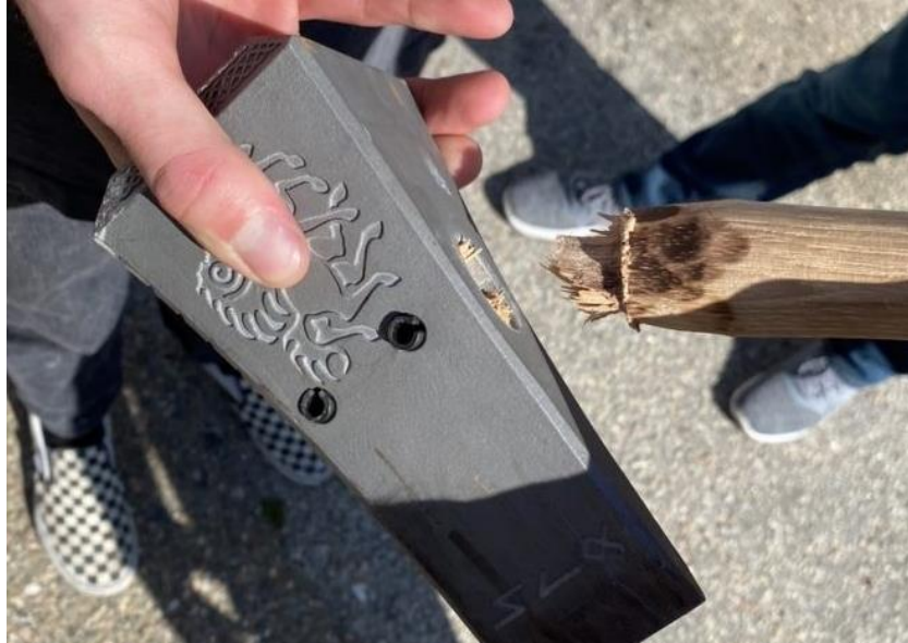
Figure 14 Effect of Roll Pins Weakening Handle
