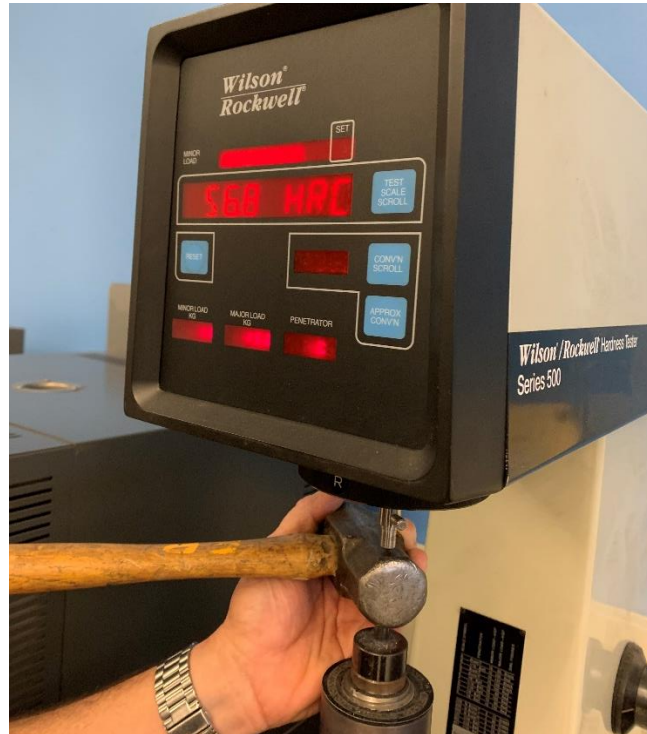
Figure 11 Rockwell Hardness Test of Other Hammers
