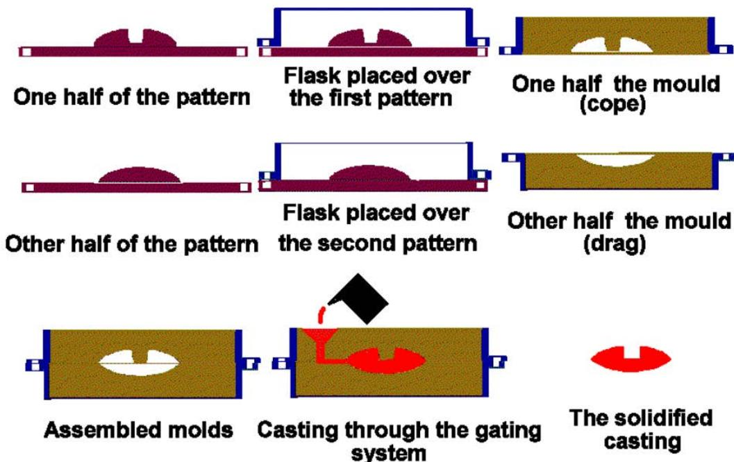
Figure 6. Basic Process of Green Sand Casting of Steels
