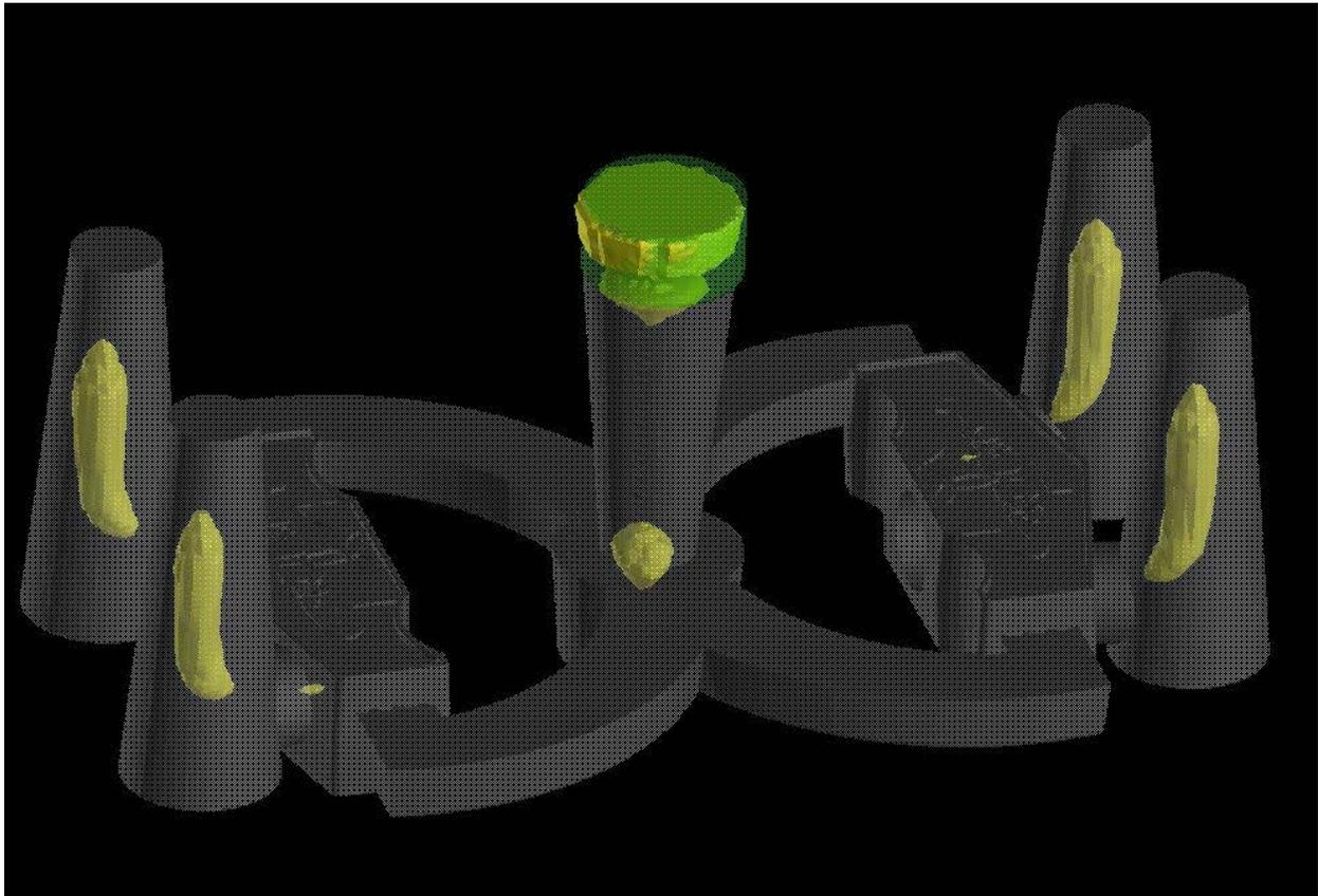
Figure 22. Final simulation of Solidcasts without little to none shrinkage.
