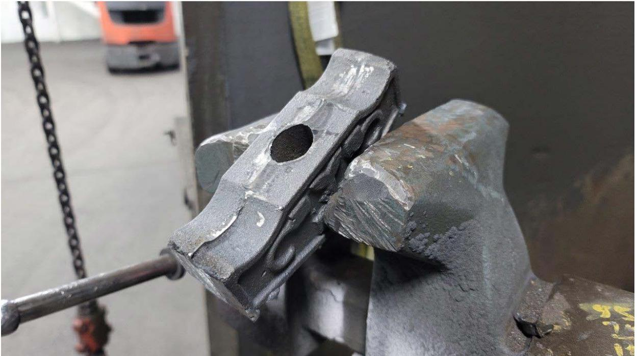
Figure 25. Hammerhead before sanding down sharp edges
