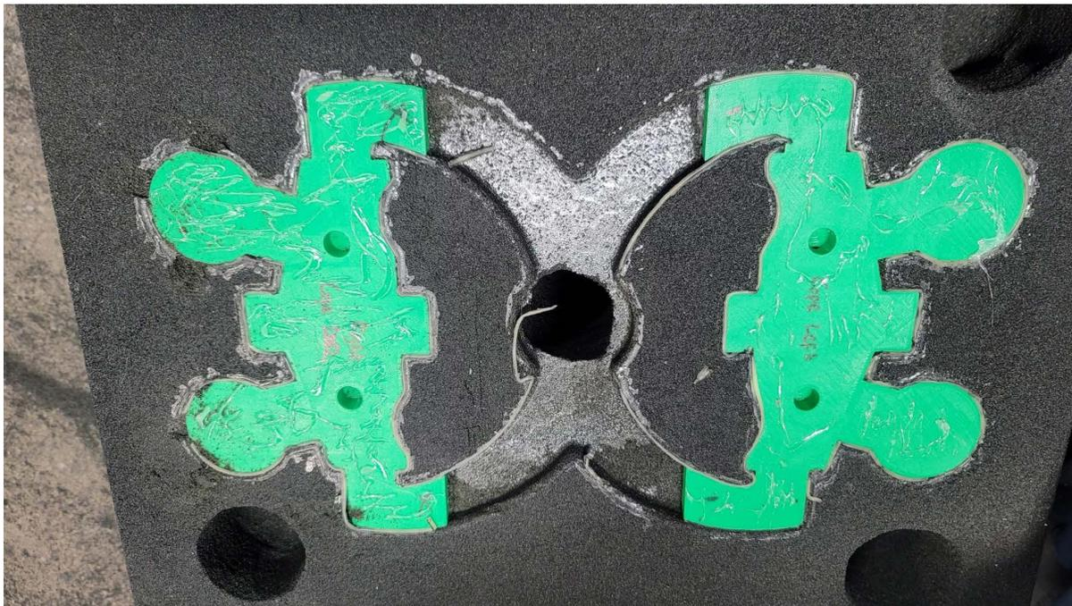
Figure 23. 3D Printed mold inserted into the sand to be used for the casting process
