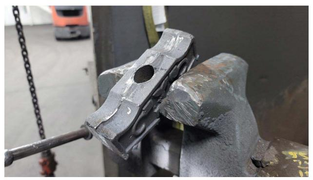
Figure 25. Hammerhead before sanding down sharp edges
