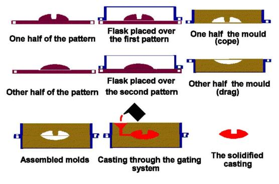
Figure 6. Basic Process of Green Sand Casting of Steels
