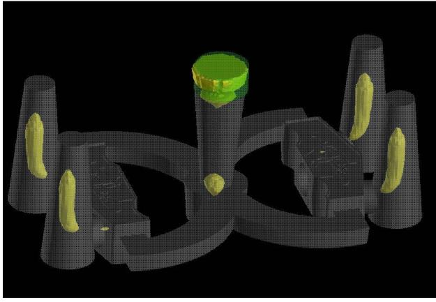
Figure 22. Final simulation of Solidcasts without little to none shinkage.
