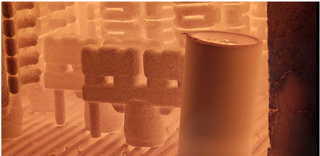
Figure 19: Preheating the mold to 1925°F before pouring
