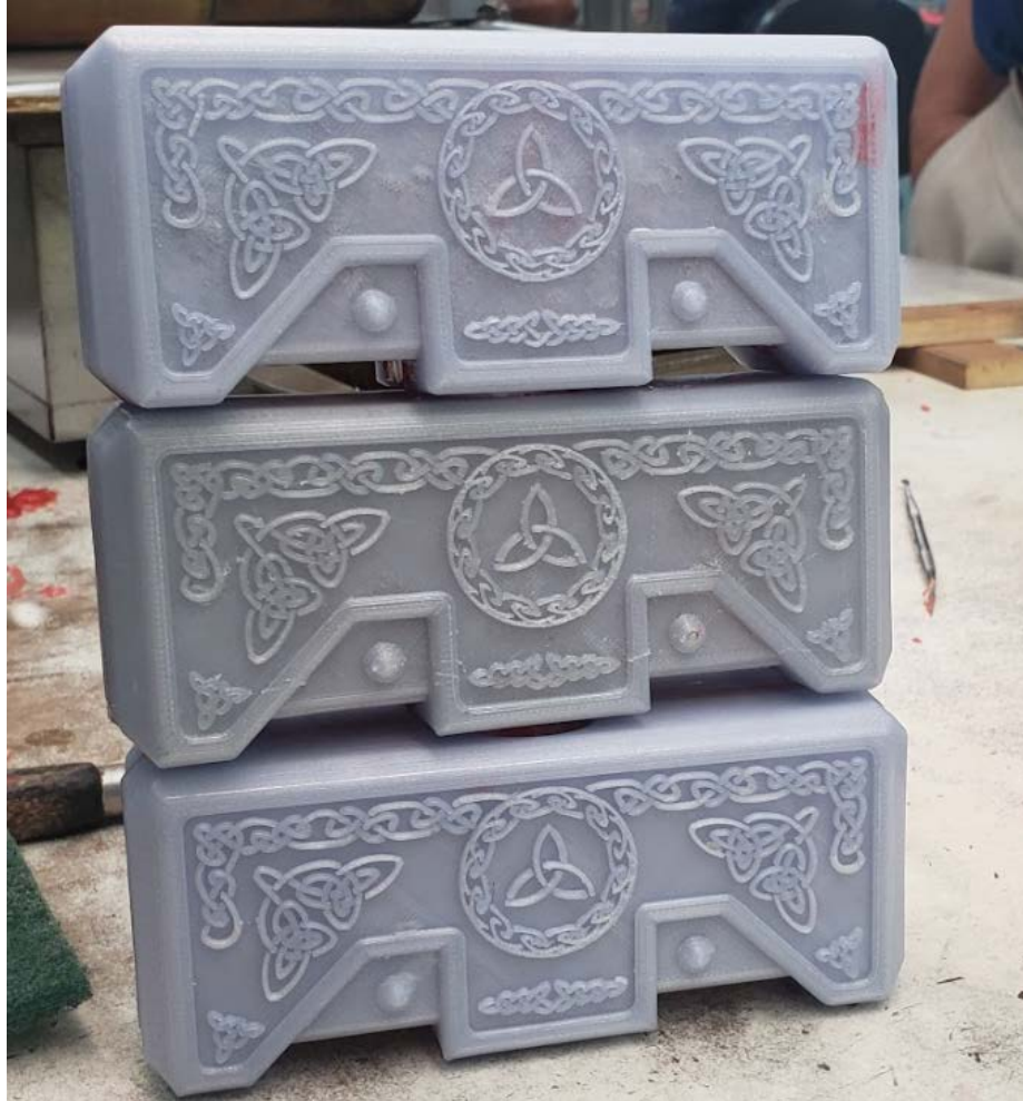
Figure 13: The top two prints are the ones print done on FlashForge with FlashPrint software.
