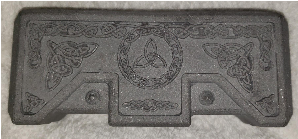
Figure 21: Final cast of one of four of the hammers with the gates removed.
