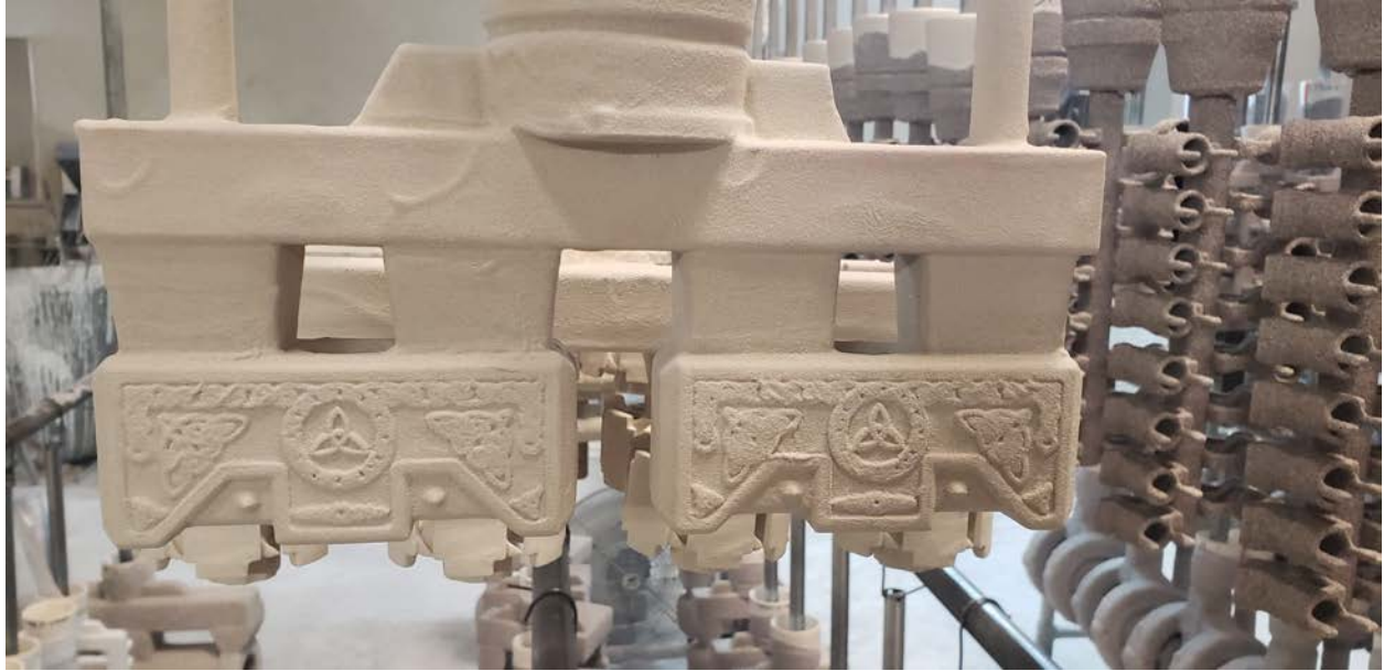
Figure 18: First layer of the ceramic shell mold of our casting.
