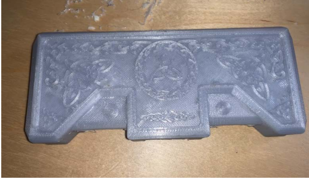
Figure 11: In this picture, one can see that this print has holes on the top surface. This would not be usable for an investment process because the slurry would seep in.
