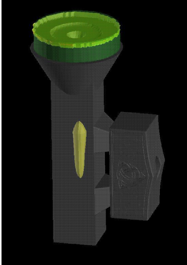
Figure 11: Shrinkage in Casting
