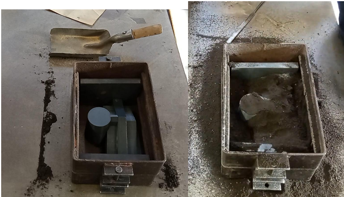
Figure 4 Sand molding down part
