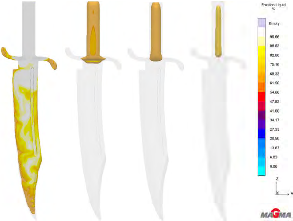
Figure 11. Solidification sequence as seen from the fraction liquid result
