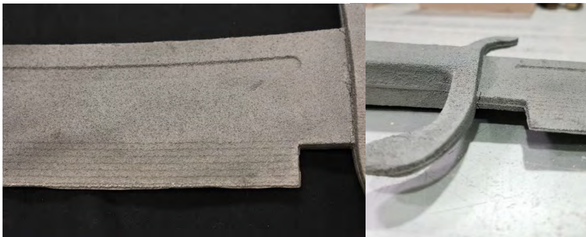
Figure 17. Hot tears developed in some of the castings. Neither of these castings appeared to have fillets around the sharp corners.
