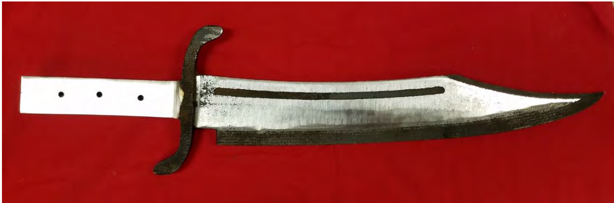
Figure 18. Knife ready for hardening and tempering.
