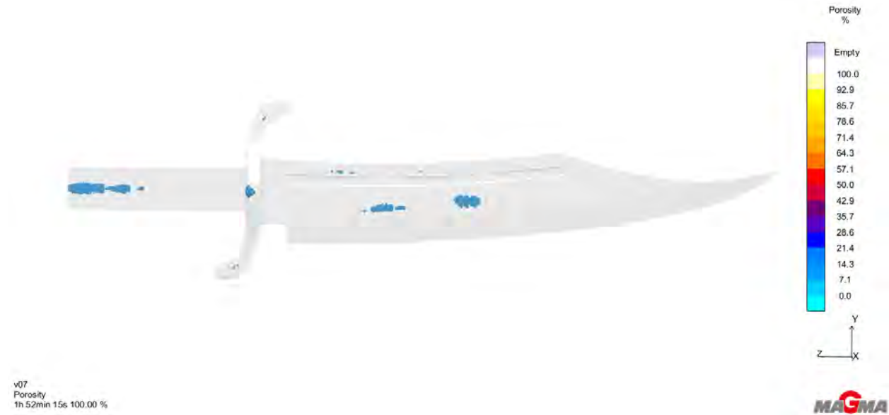
Figure 29. Porosity results for the complete knife; note that there are numerous areas of concern on the blade but these are generally in thick areas.
