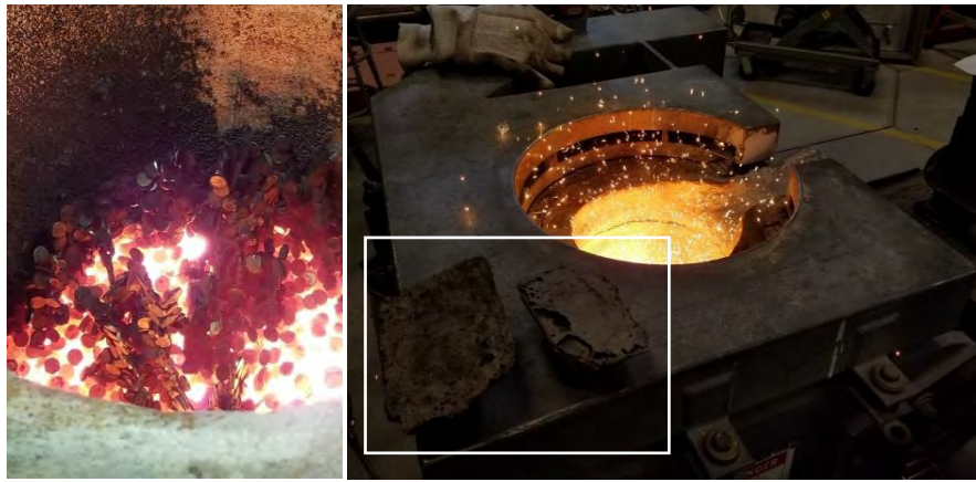
Figure 3. Melting process; left: base steel charge, right: carbon boil (rectangle shows the Sorelmetal®)
