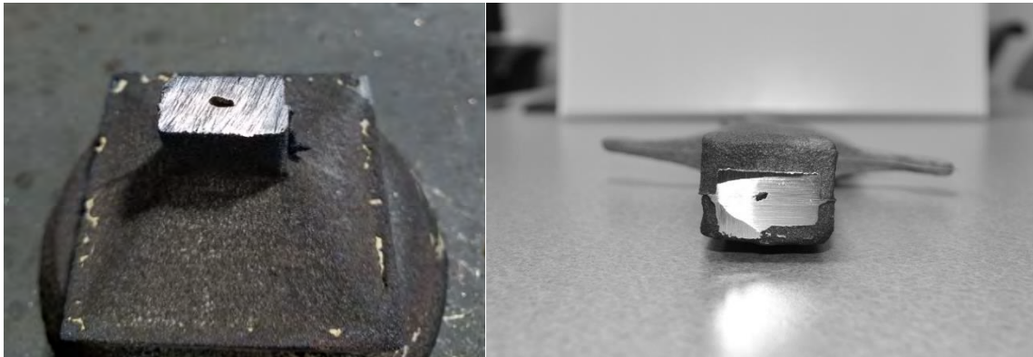
Figure 16. Cross-sectional view showing centerline porosity
