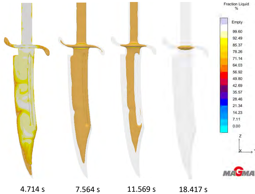
Figure 8. Fraction liquid fringe plots at different times. X-ray scale set such that any volume with less than 70% liquid is hidden from view.
