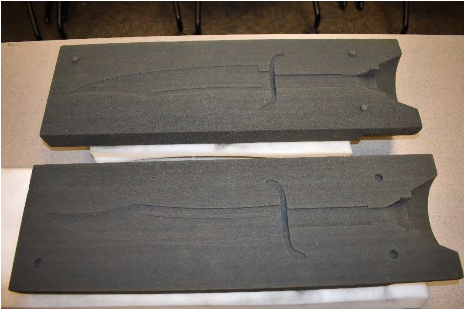
Figure 6. Additively manufactured two-piece sand mold courtesy of ExOne
