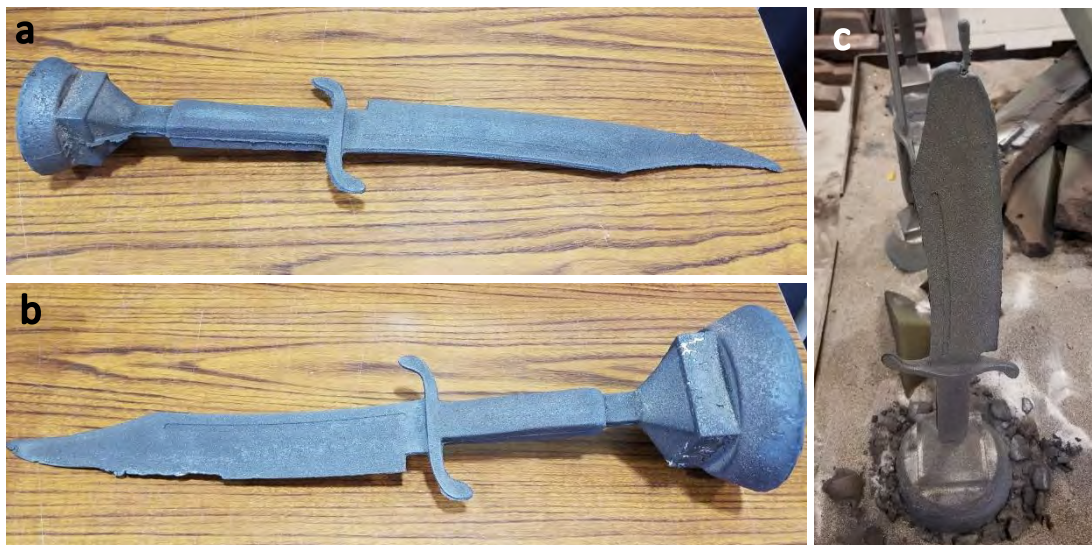
Figure 15. As-cast knives showing different outcomes: a) complete fill without filter, b) incomplete fill with filter, and c) incomplete fill due to low pouring temperature.
