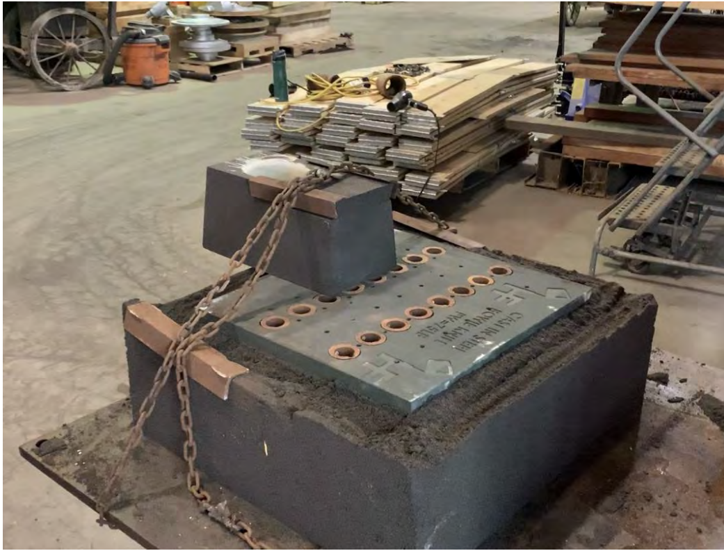
Figure 37. Mold Before Casting
