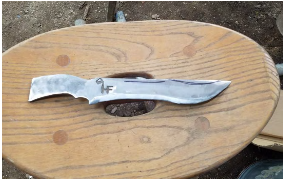
Figure 17. Pre- Heat-Treated Blade
