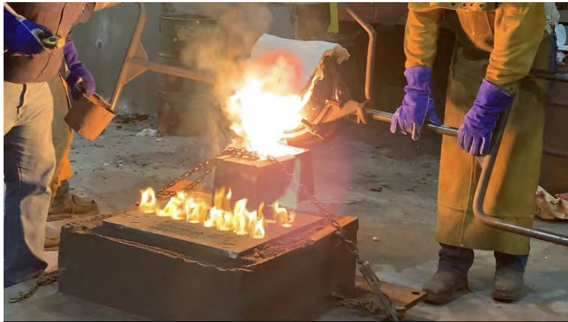
Figure 8. Casting of the Bowie Knife
