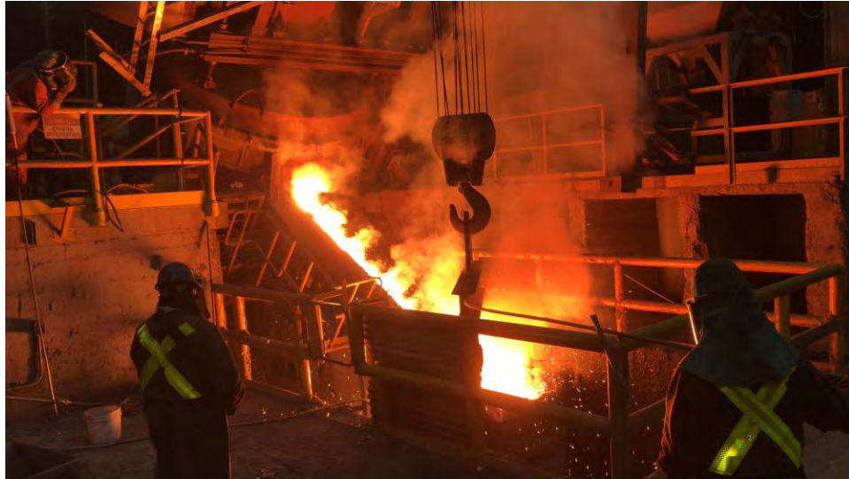
FIGURE 15: MOLTEN METAL DURING POUR FOR BOWIE KNIFE CASTING
