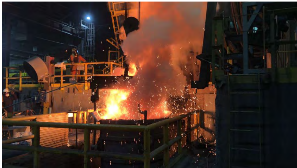
FIGURE 15: MOLTEN METAL DURING POUR FOR BOWIE KNIFE CASTING
