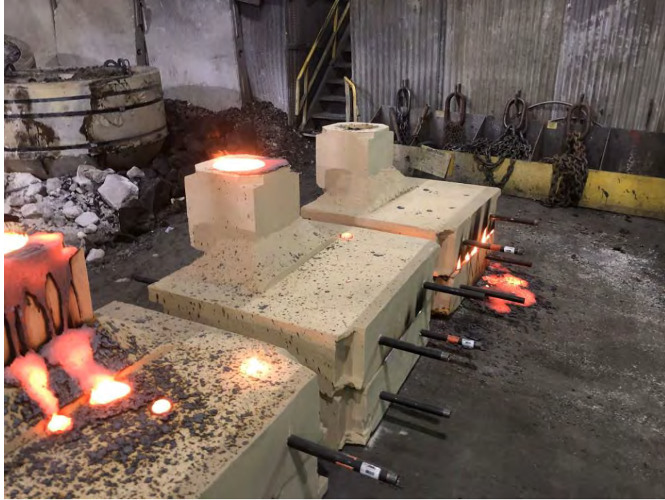
FIGURE 18: SEPARATION FAILURE OF COPE AND DRAG
