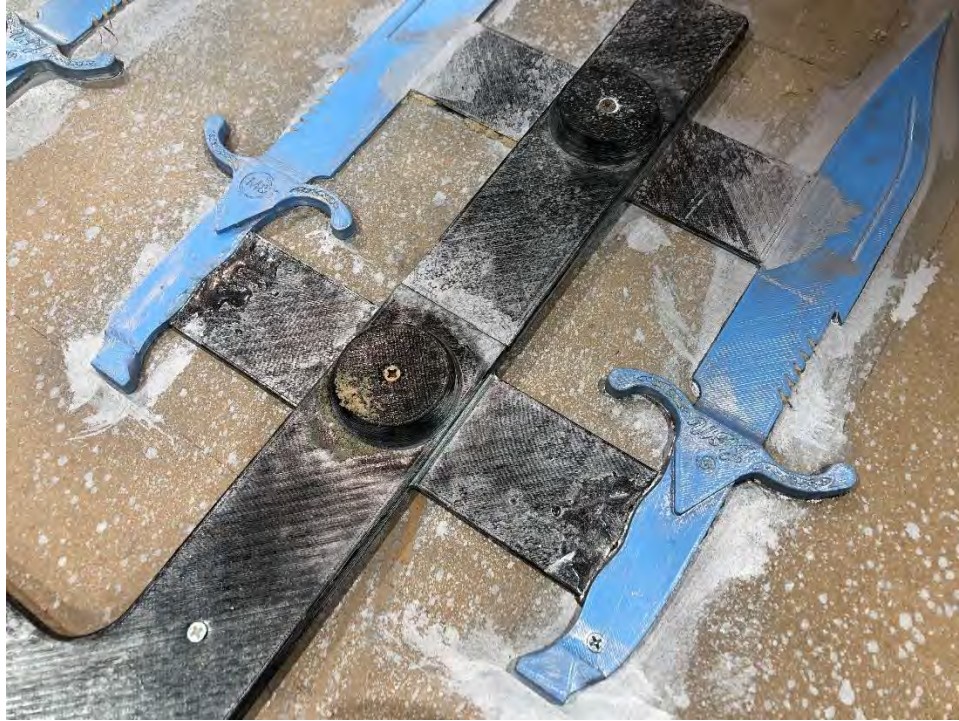
FIGURE 11: INSTALATION OF PUTTY ANDEXPOXY ON PATTERN TO SEAL GAPS
