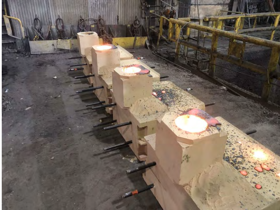
FIGURE 17: FOUR MOLDS USED IN CASTING POUR
