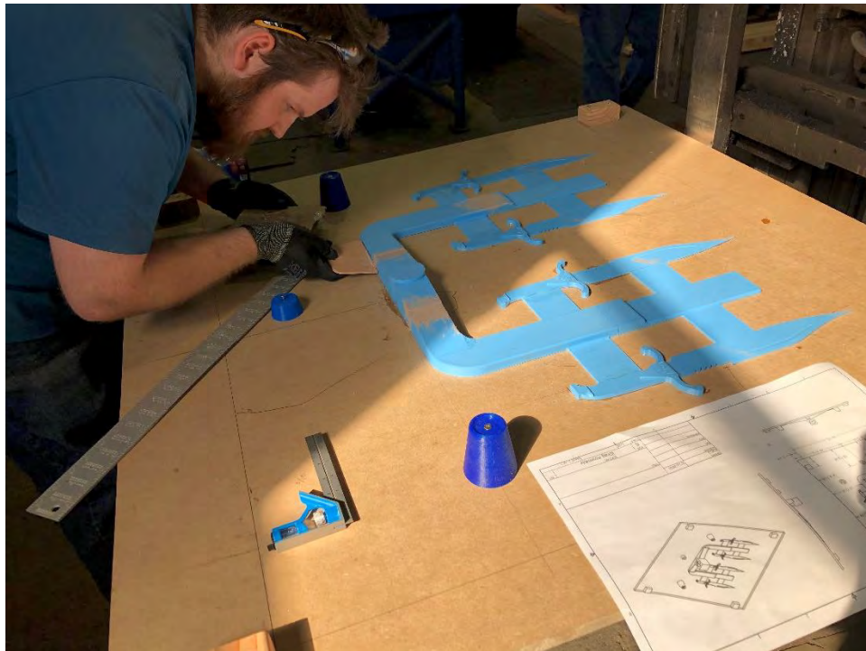
FIGURE 10: INSTALATION OF 3D PRINTED PATTERN TO MOLD PLATE
