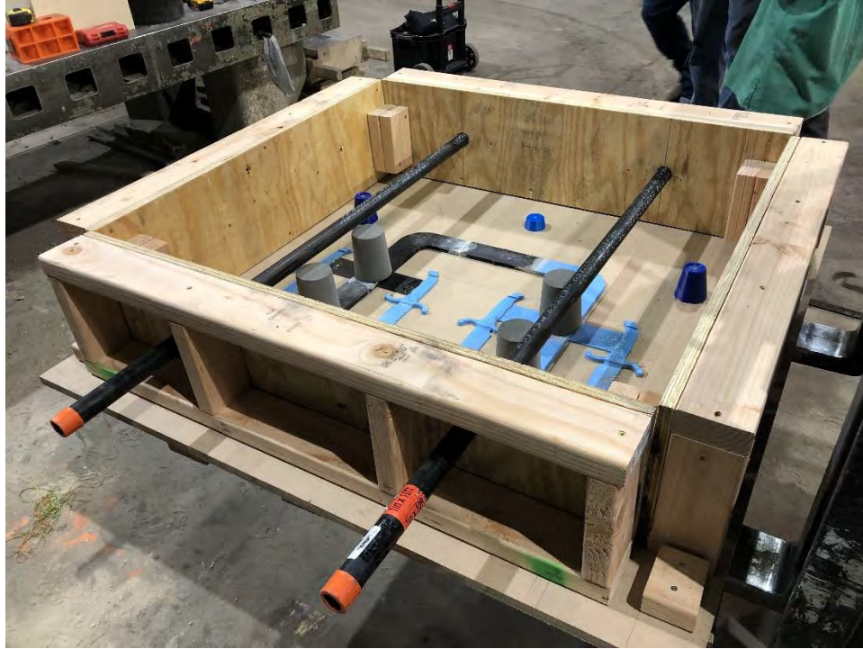
FIGURE 12: MOLD SETUP PRIOR TO ADDING SAND
