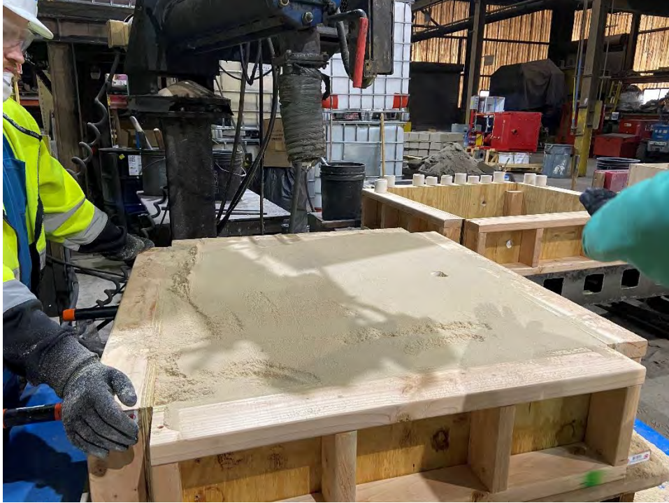
FIGURE 13: MOLDHALF PACKED WITH SAND
