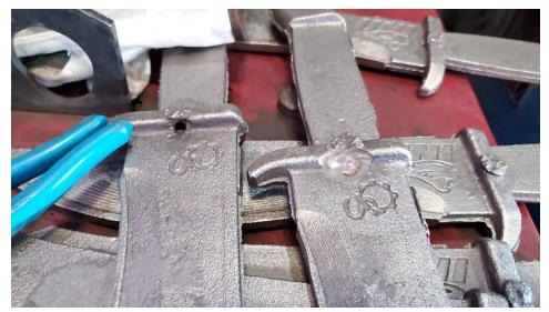
Figure 9. The shrink defect is shown before and after welding. (but before the weld was dressed)
