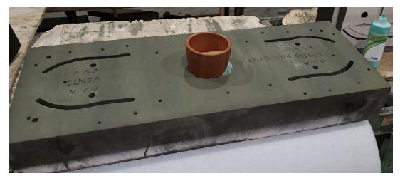
Figure 5. Modifications to the mold such as larger pour cup and vents can be seen above.
