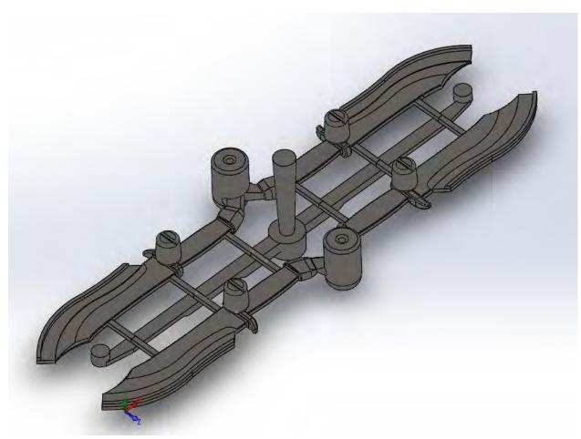
Figure 3. The image above shows the final knife design with rigging
