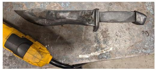
Figure 10. After grinding, the knife is near final shape.
