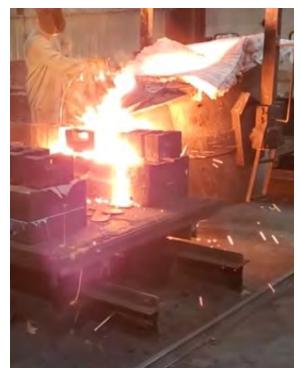
Figure 7. A bowie knife mold being poured at Omaha Steel is shown.
