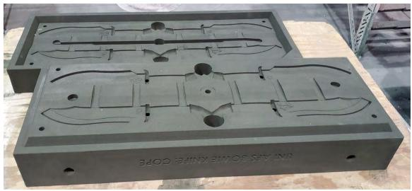
Figure 4. Above is a picture of the 3d printed mold
