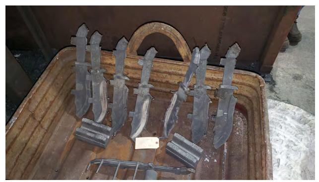
Figure 8. Raw castings after degating are shown.
