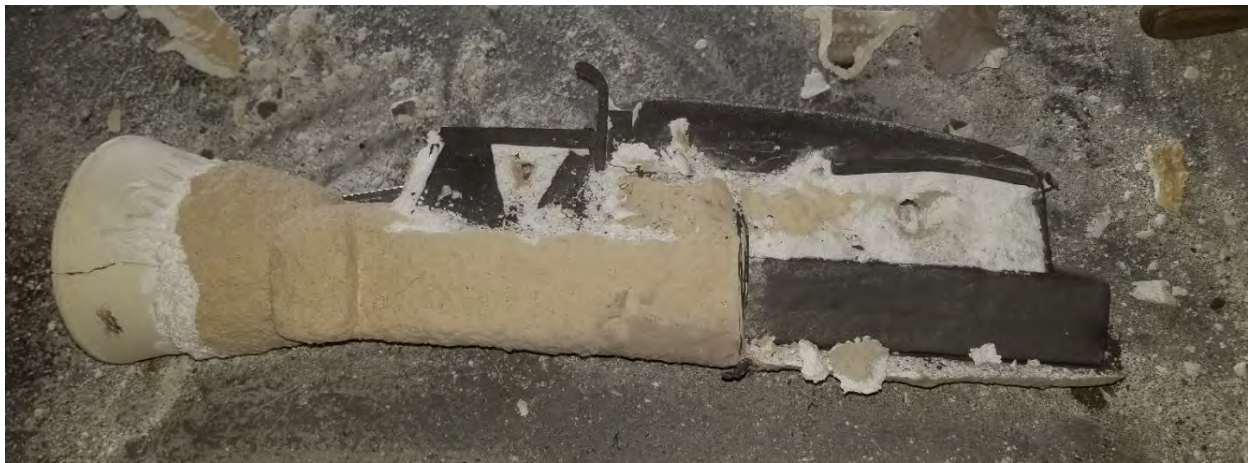
Figure 11. 440c Bowie Knife partially demolded.
