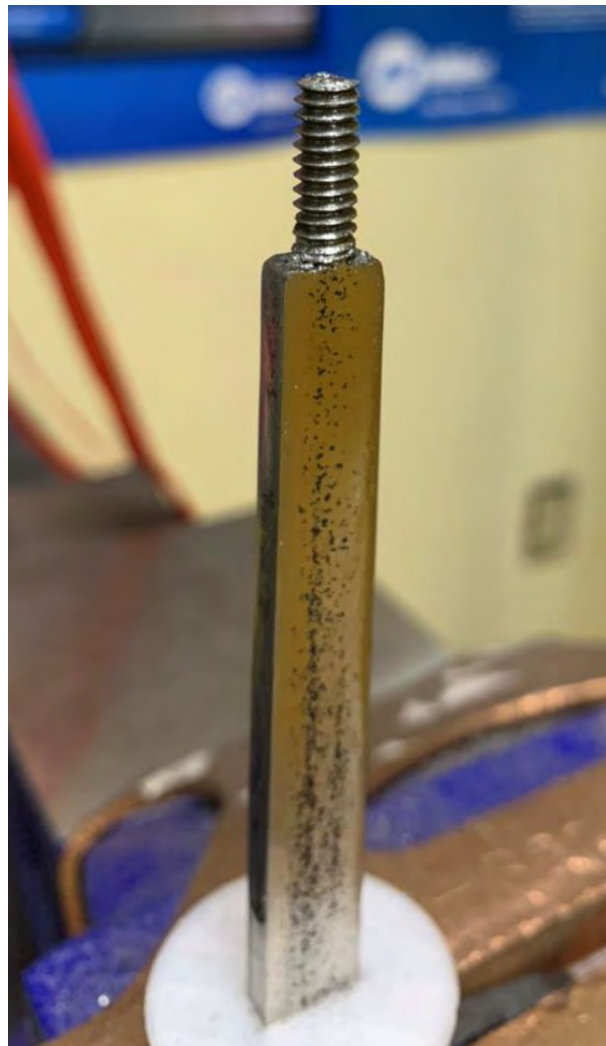
Figure 15. Threaded extension on pommel.
