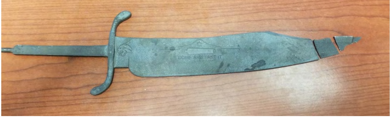
Figure 10. D2 Steel Bowie knife broken tip after straightening.
