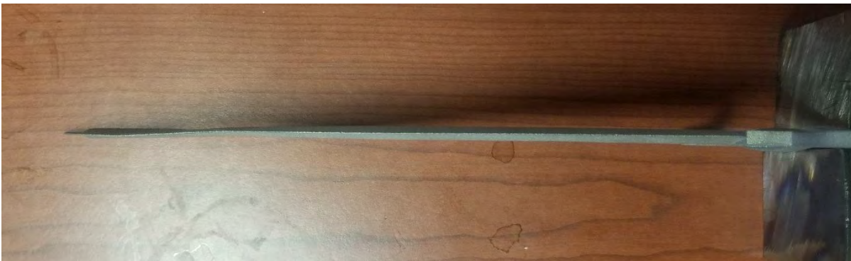
Figure 9.c. Warp in D2 Steel Bowie knife post degating process.
