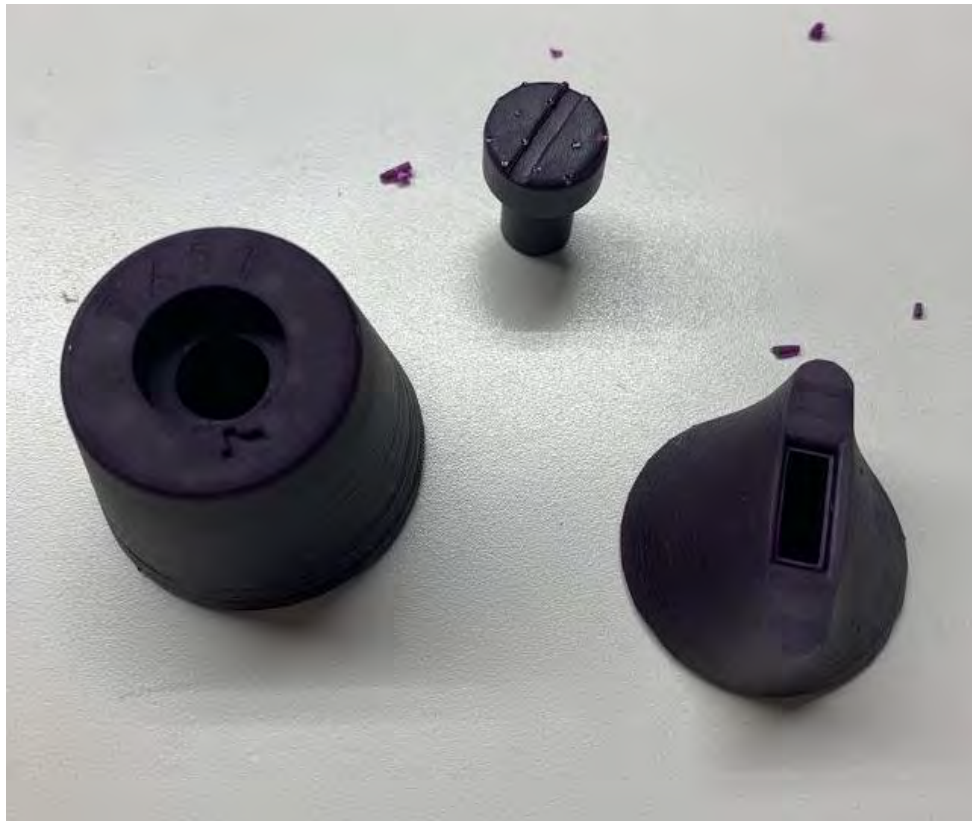
Figure 17. 3D wax printed pommel, brass joint, and screw.
