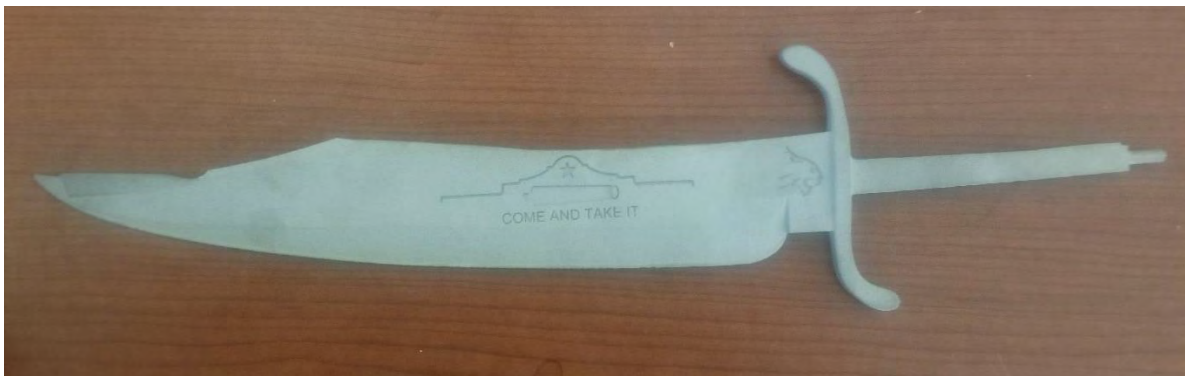
Figure 9.b. Chip in D2 Steel Bowie knife post degating process.
