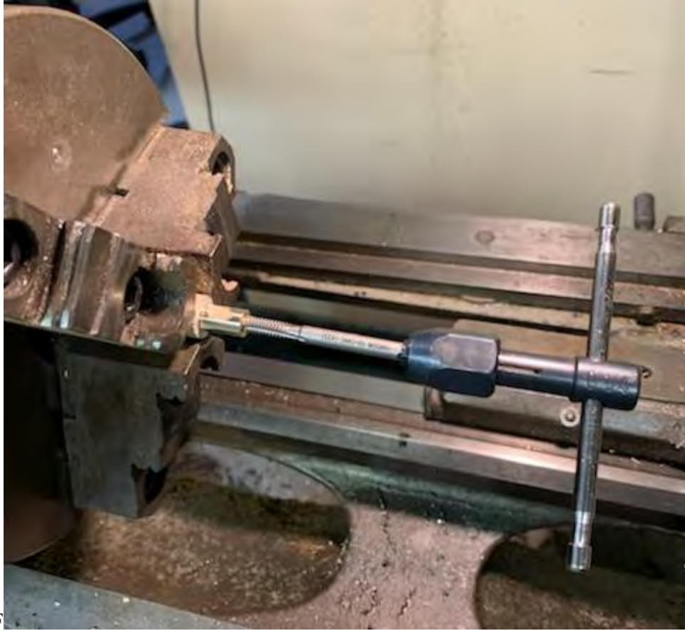
Figure 19. Threading process of screw in pommel assembly.
