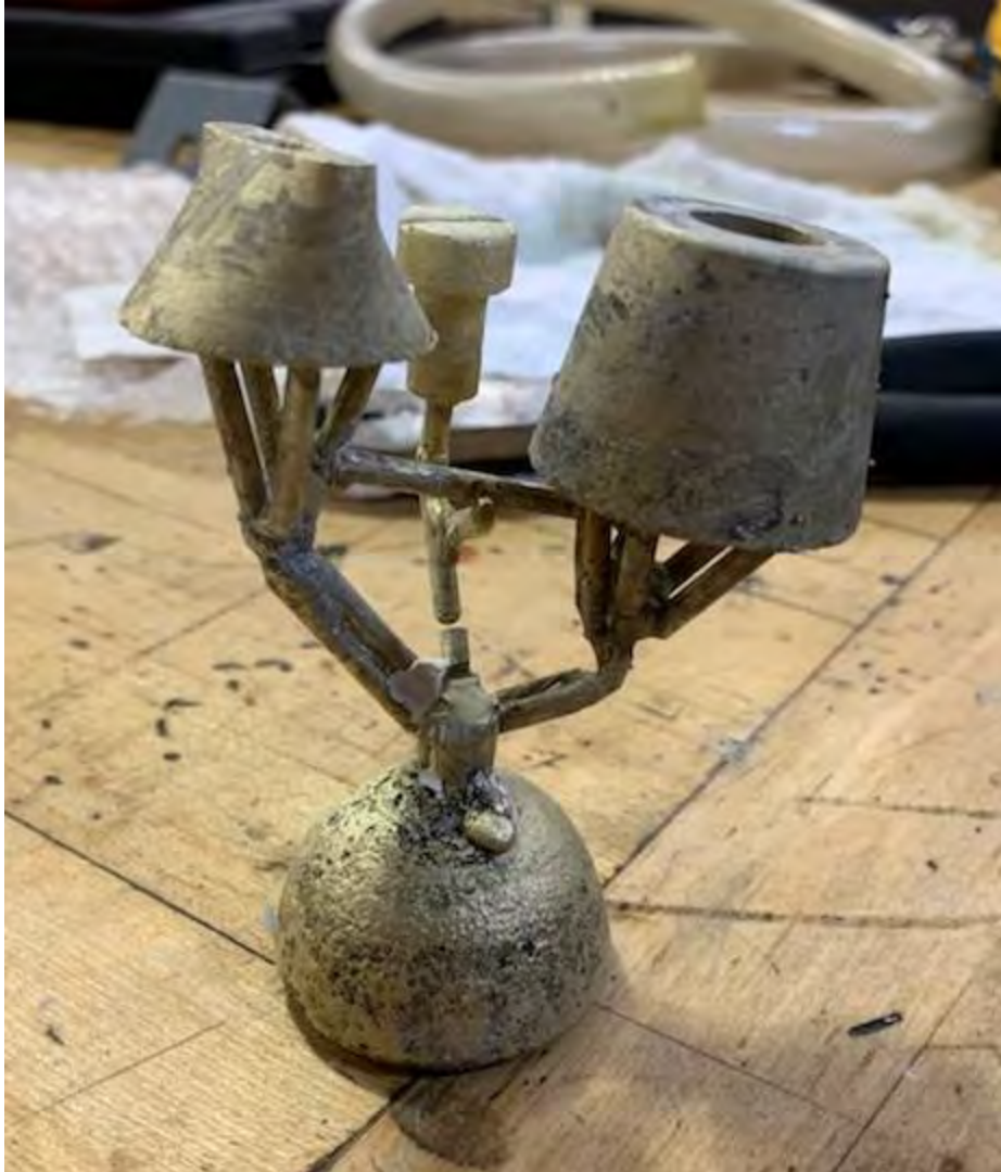
Figure 18. Casting of pommel, brass joint, and screw.
