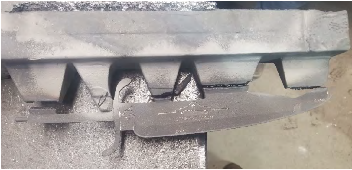
Figure 9.a. Chip in D2 steel Bowie knife during degating process.
