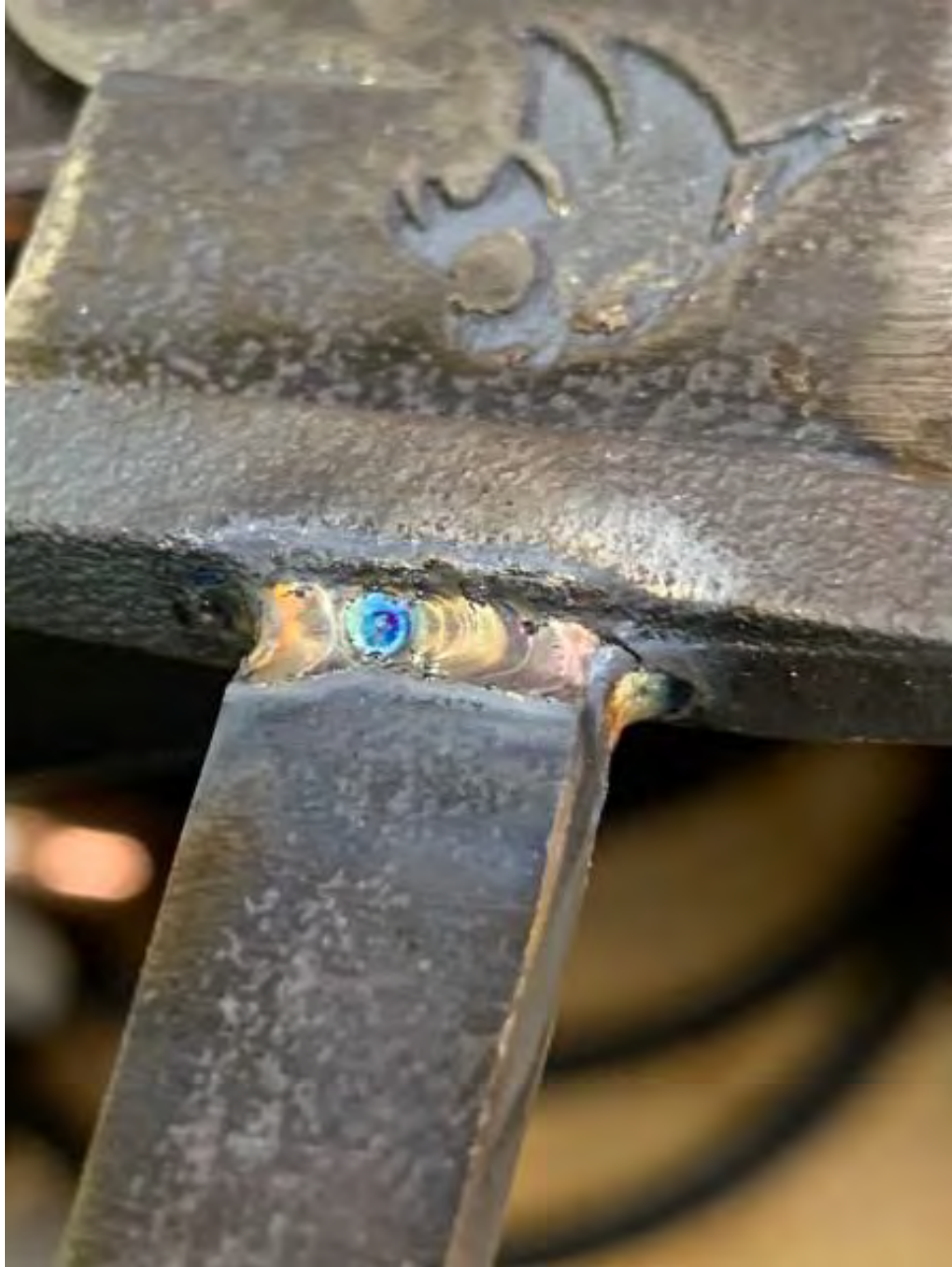
Figure 21. TIG repair of tang.
