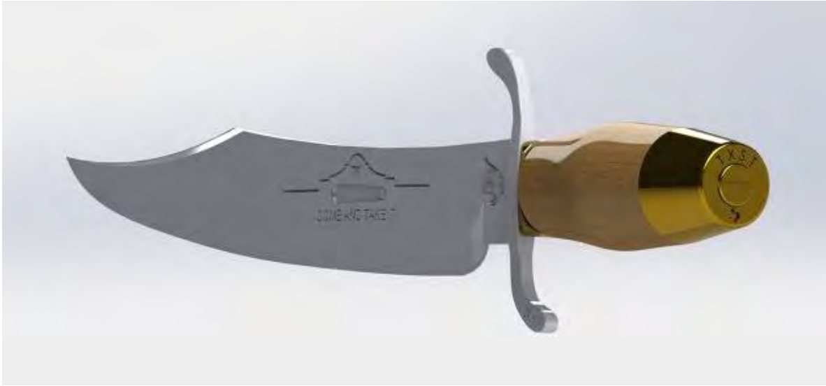
Figure 16. 3D modeled version of handle and pommel assembly.
