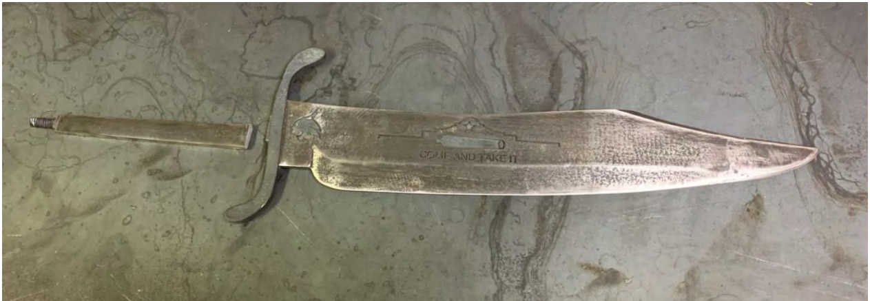
Figure 20. Broken tang during assembly.
