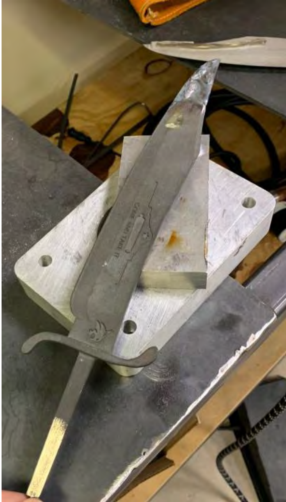
Figure 13. Tip of D2 steel knife TIG welded together.
