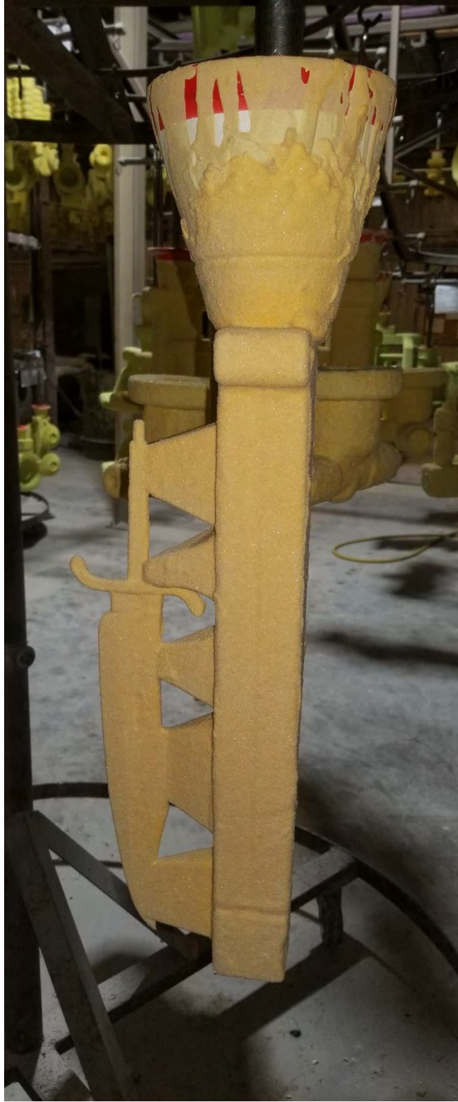
Figure 8. Mold of Bowie knife prepared and ready for investment casting.
