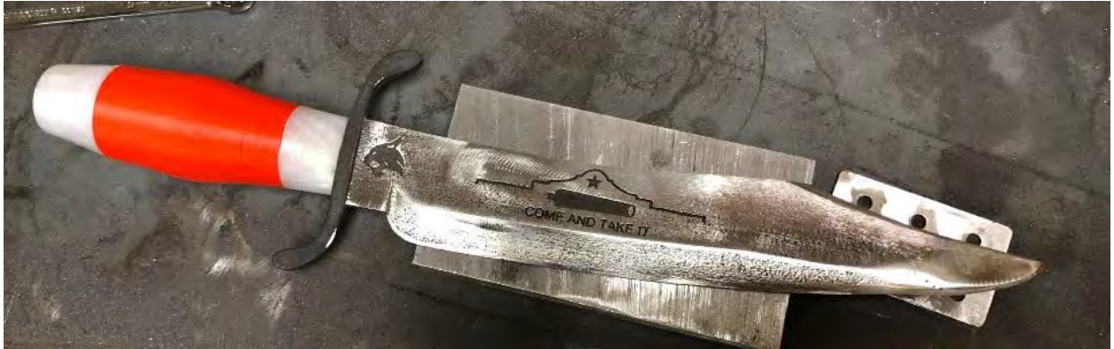
Figure 14. Weld ground flush with surface of D2 steel Knife.
