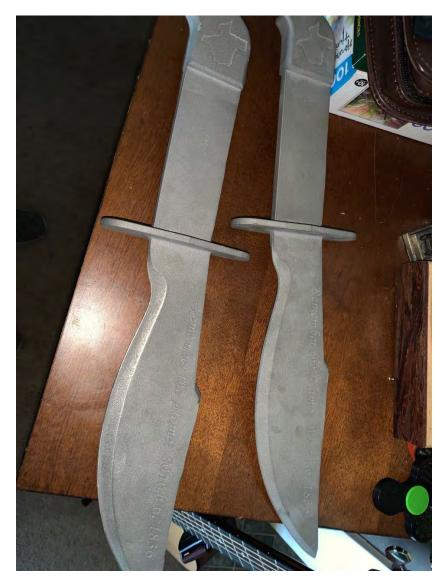
Figure 8: Raw Bowie Knife Castings received from AFG
