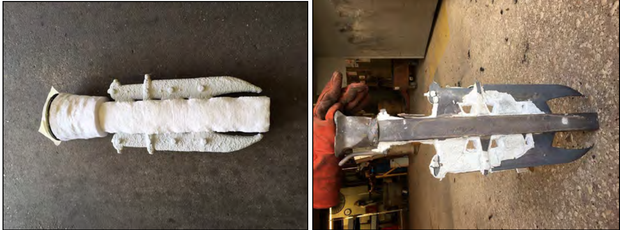
Figure 11. Ceramic shell of our casting tree (left), Final cast of one of our casting trees after being shook out (right)
