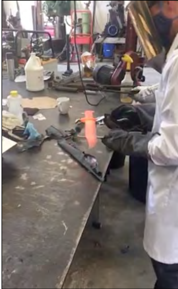
Figure 16. Removal of the knife from the heat treatment steel foil wrapping
