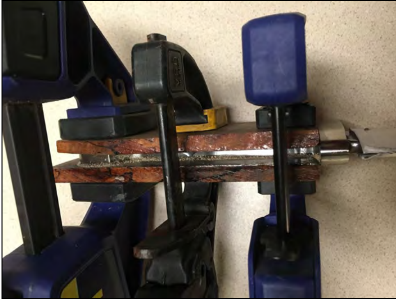
Figure 18. Epoxying the spalted pecan wood to the handle
