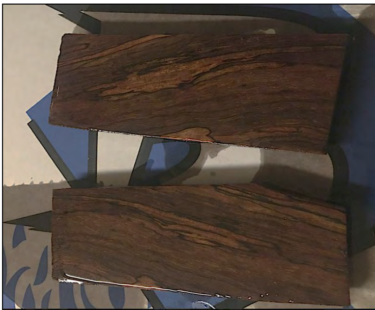
Figure 15. Our spalted pecan wood curing after being soaked in polyurethane
