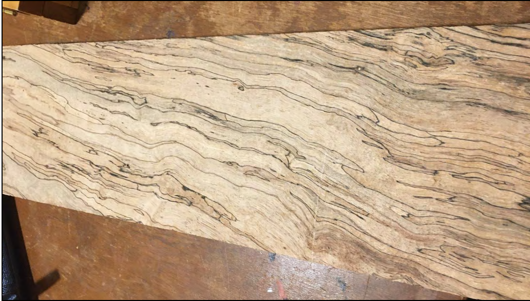
Figure 14. Sample of spalted pecan wood used for the handle
