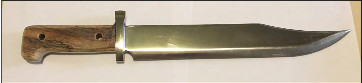
Figure 20. Overall view of the handle before epoxying the pins in place
