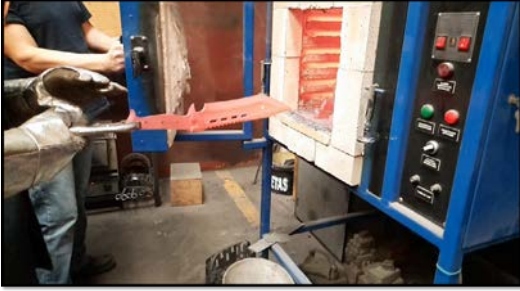
Figure 22. Bowies removed from the furnace to be quenched
