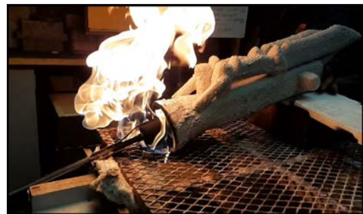
Figure 13. The wax is melted and drained
