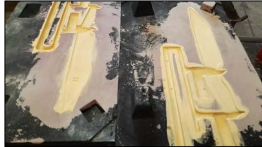
Figure 16. Cope and drag molds washed with zircon wash coating
