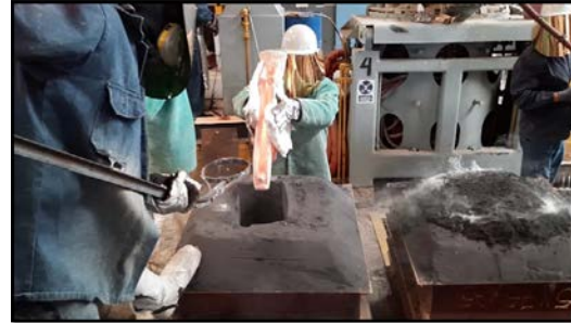
Figure 20. Shell placed to be poured
