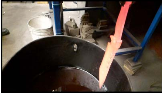
Figure 23. Blades quenched in oil
