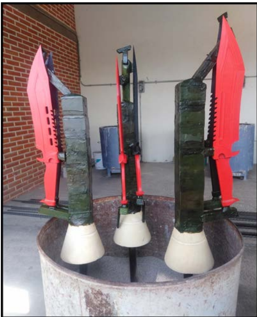
Figure 12. Two PLA patterns put together in one shell
