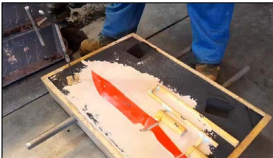
Figure 15. No-bake mold faced with ceramic sand.
