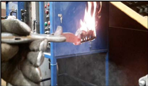
Figure 24. Bowies after quenched in oil. Note that only the blade was quenched
