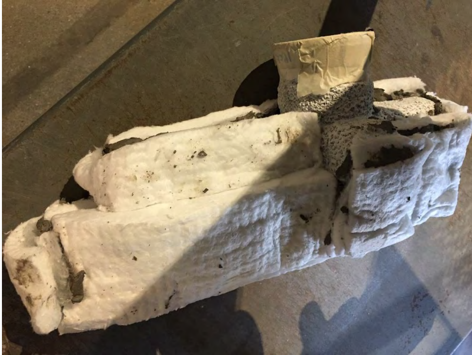
Figure 28: Cleaned and Insulated Mold
