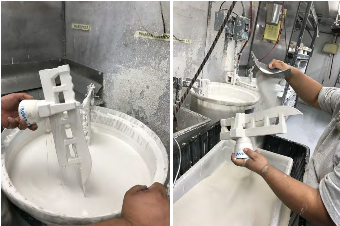
Figure 22: Initial Slurry Coating
