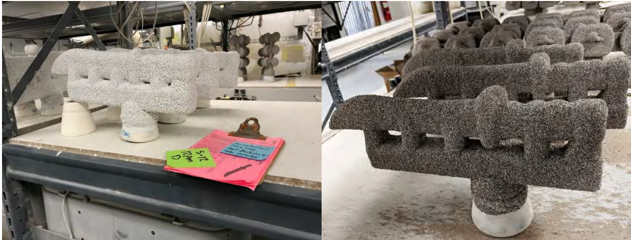
Figure 24: Dry Slurry Coating
