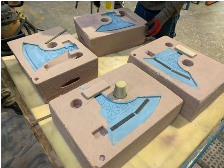
Figure 5. The molds coated with a high solid zircon coating.
