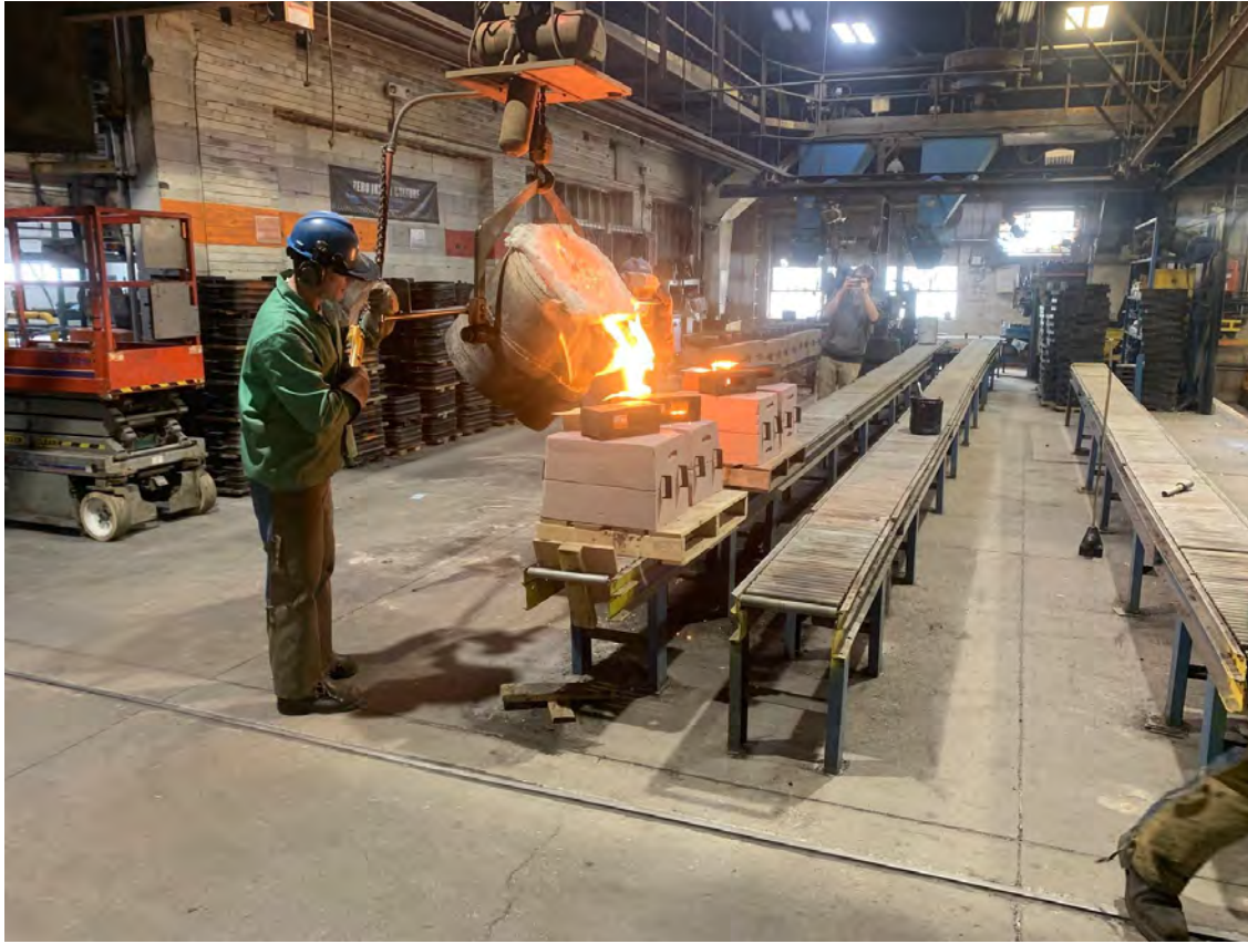
Figure 6. The pouring of the Axe heads.
