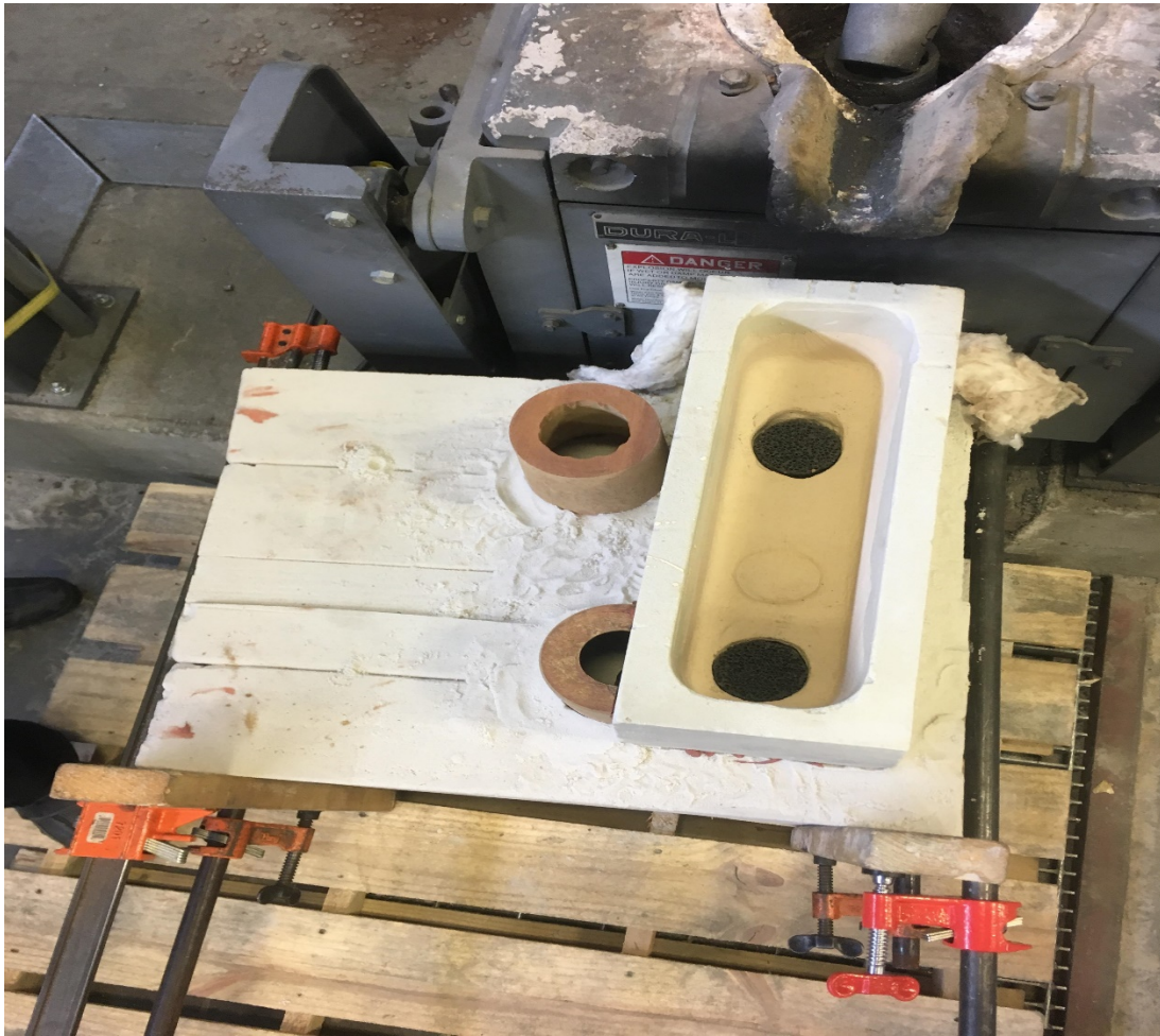
Figure 14 Set up of molds pre-cast
