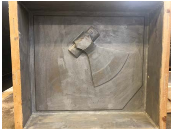
Figure 13 CNC'ed pattern boxes used to make sand molds
