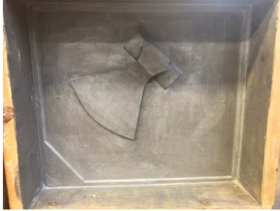
Figure 12 CNC'ed pattern boxes used to make sand molds
