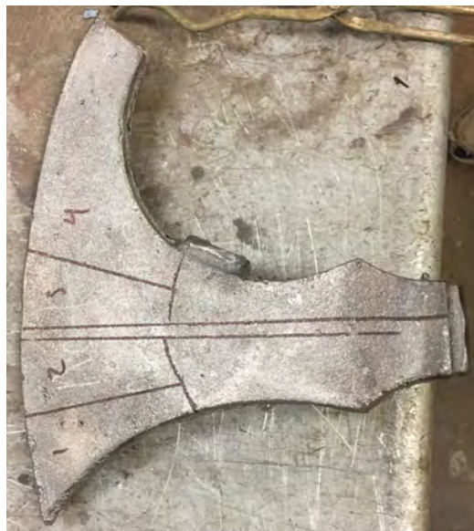
Figure 03: Photograph of the axe sectioning pattern for various heat treat attempts.
