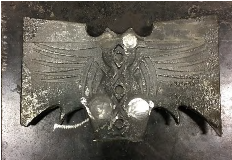
Figure 30. Axe Head Ready for Heat Treat
