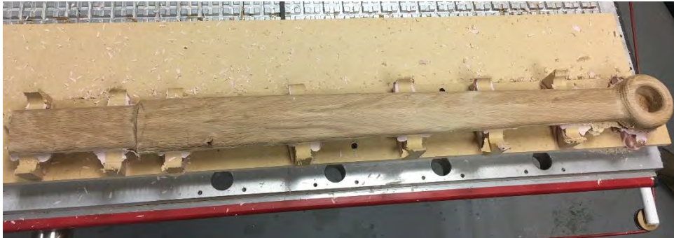
Figure 34. Second side of the axe profile machined.
