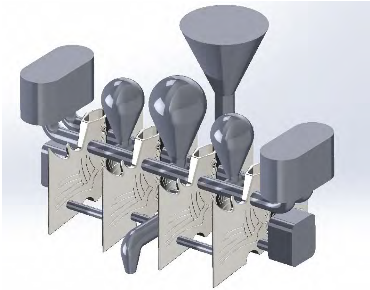
Figure 16. Final Gating Design
