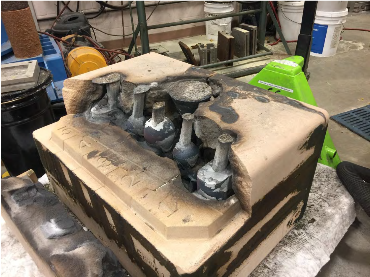
Figure 26. Mold After two days of cooling
