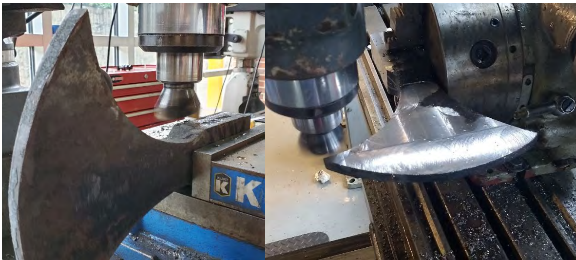
Figure 11: Planing faces of axe (left), milling cheeks (right)
