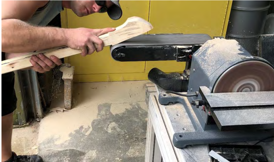
Figure 18: Sanding final contours of the handle
