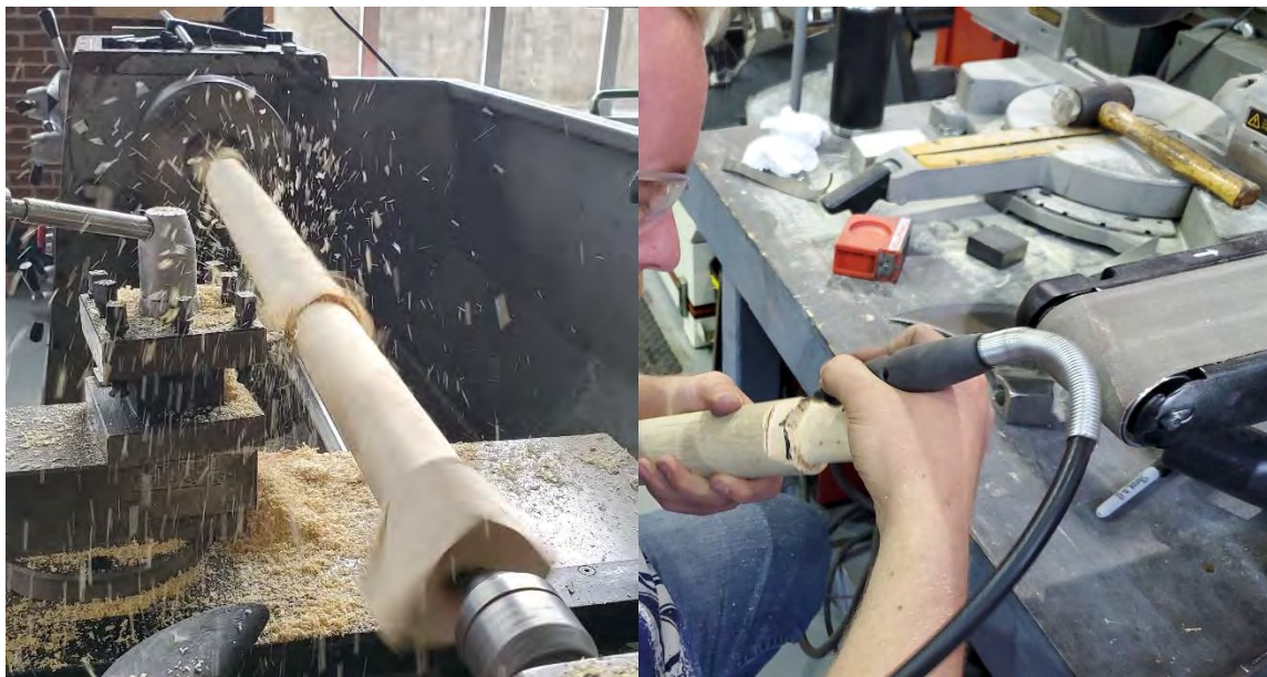
Figure 17: Haft machining on lathe (left), making eye and shoulder (right)
