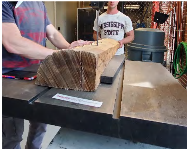
Figure 16: Cutting the haft material from a hickory log
