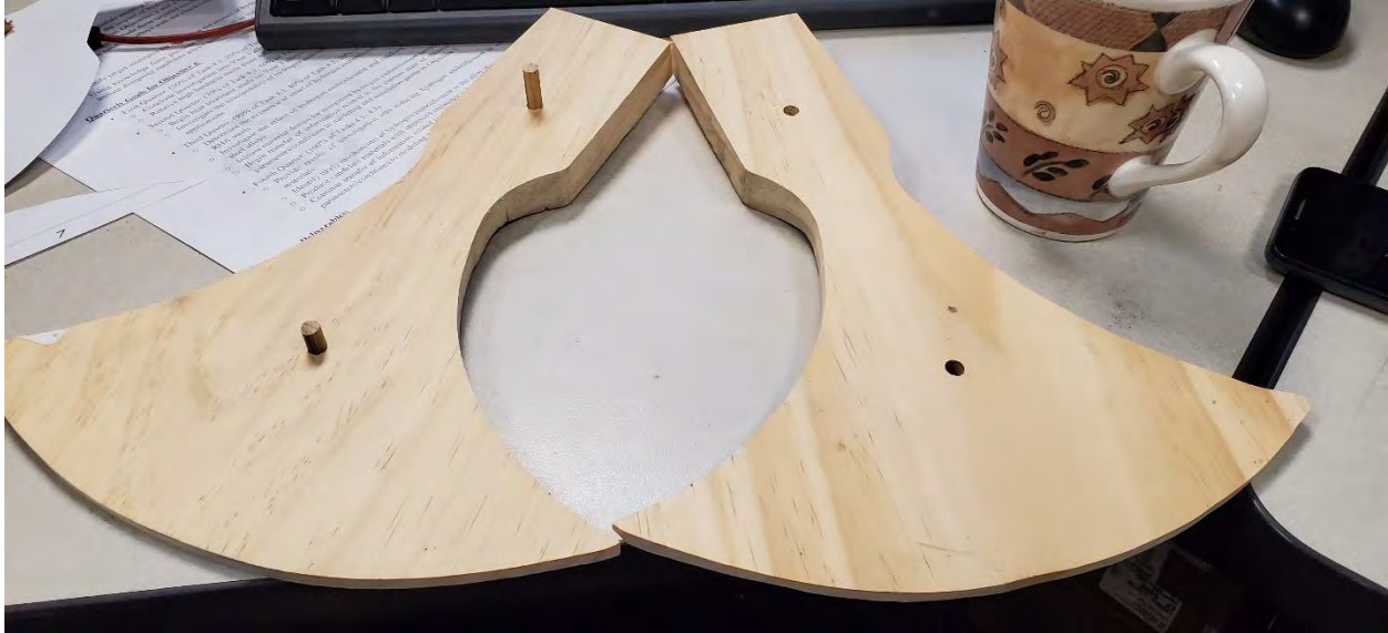
Figure 6: Split positive pattern with dowel pins
