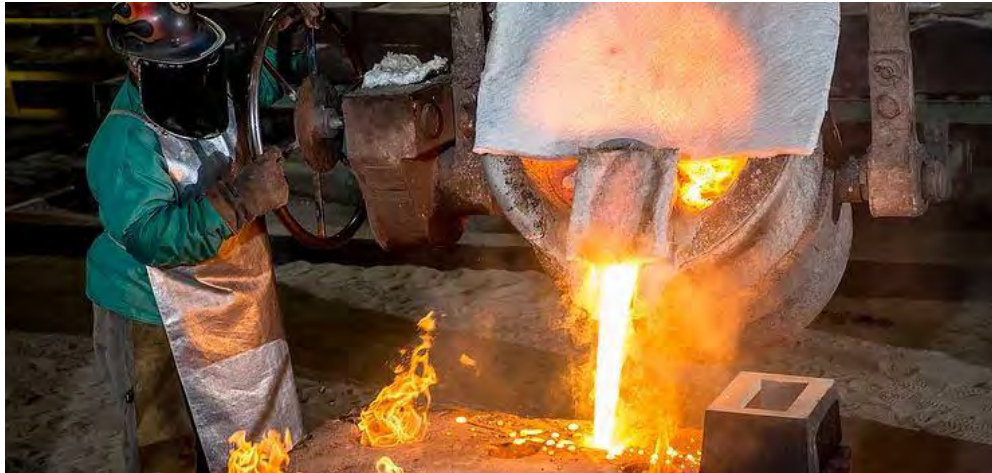
Figure 9: Pouring into a mold at SCP [7]
