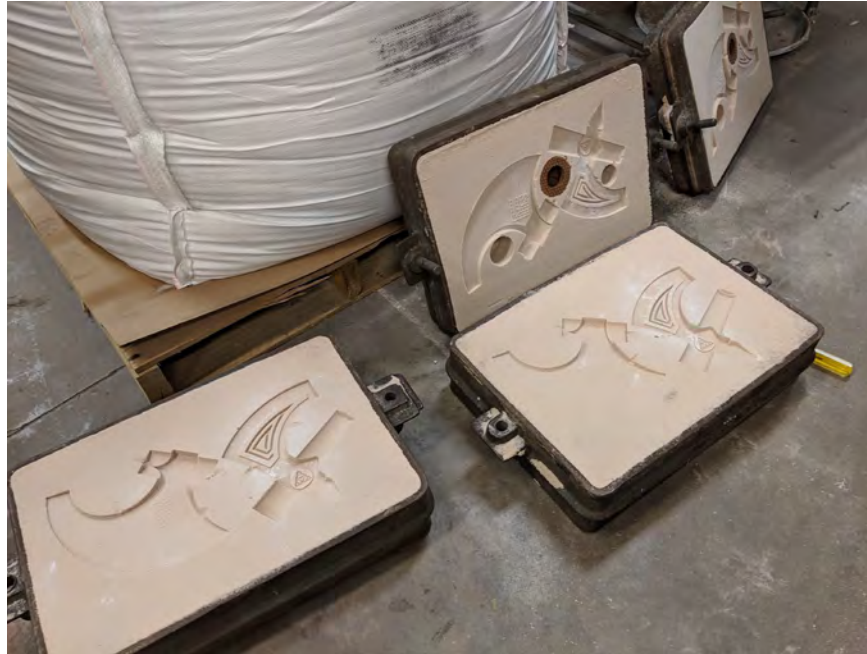
Figure 6. Completed axe head mold using chemically bonded AFS60 silica sand
