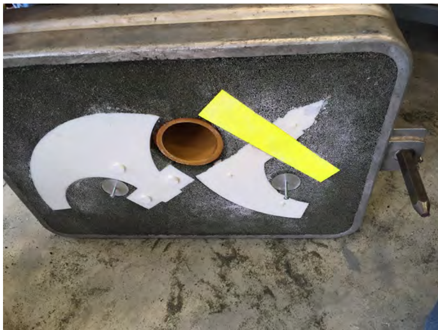
Figure 5. Completed chemically bonded sand mold before removing the patterns and risers
