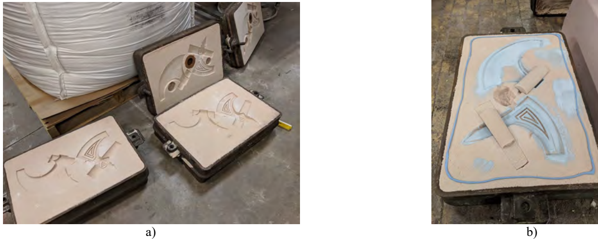
Figure 17: a) Molds made at Missouri S&T b) Mold with zircon wash to minimize metal-mold interaction
