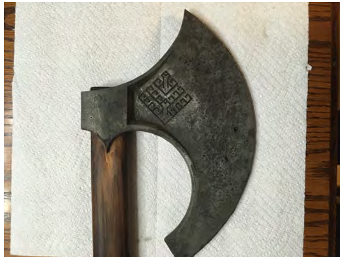
Figure 16: GIW Casting with Large Amounts of Surface Porosities
