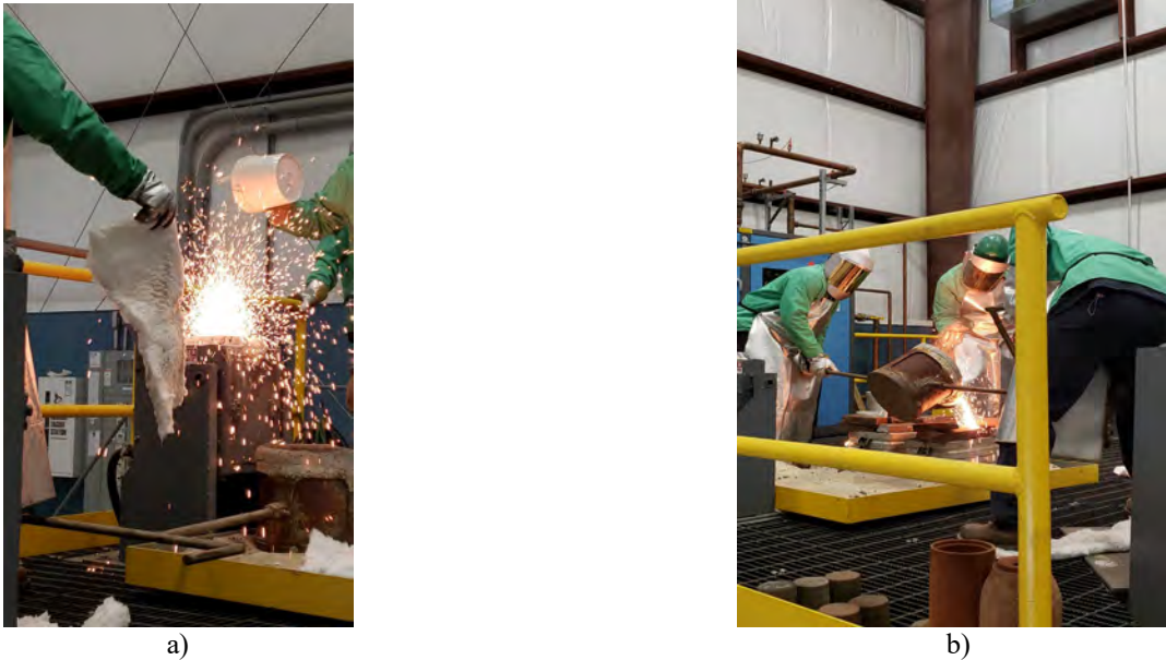
Figure 15: a) Ferrous alloys were poured into the furnace to achieve correct composition b) Pouring of molten steel into molds
