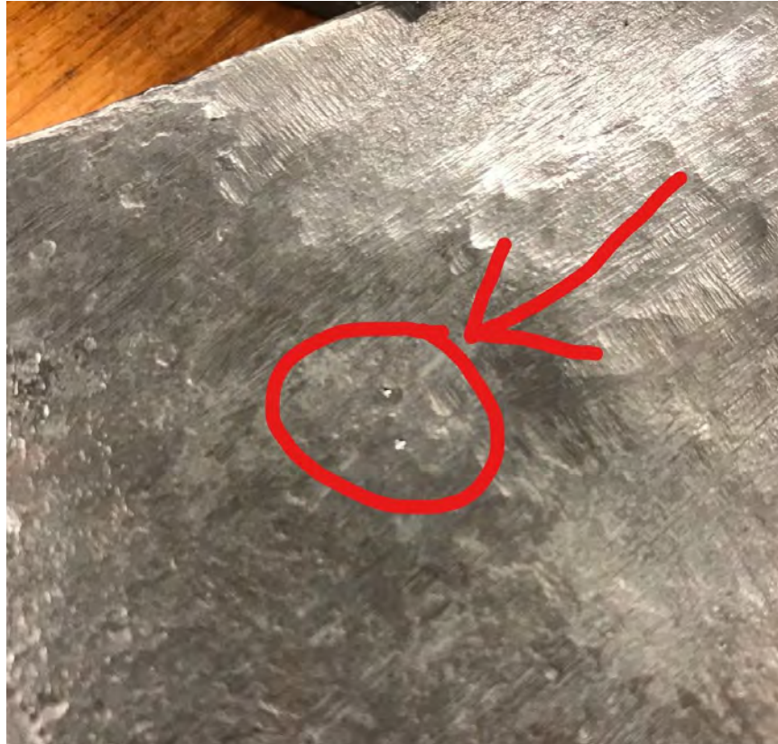
Figure 34: Post heat treatment hardness testing - HRC 28
