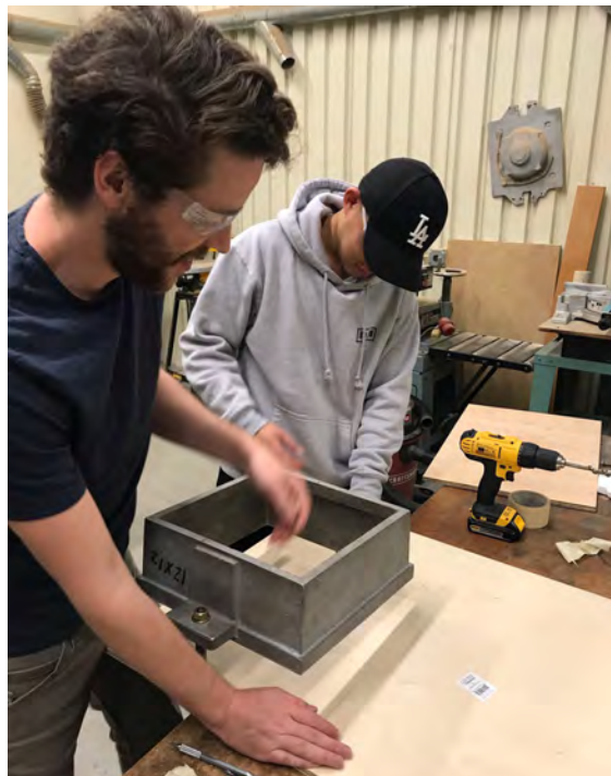
Figure 23: Steven and Ben drilling holes into matchplate.
