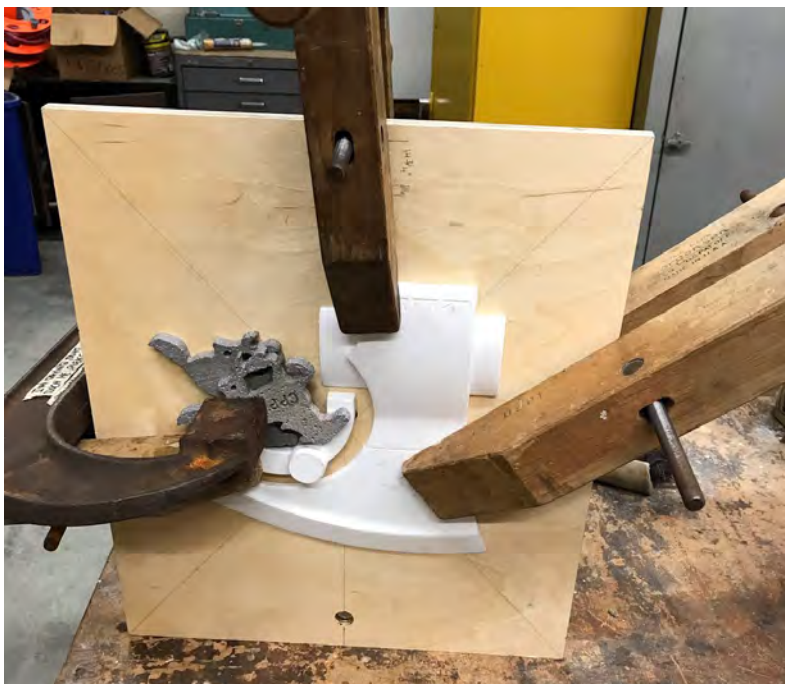
Figure 25: Clamping cope and drag patterns for glueing
