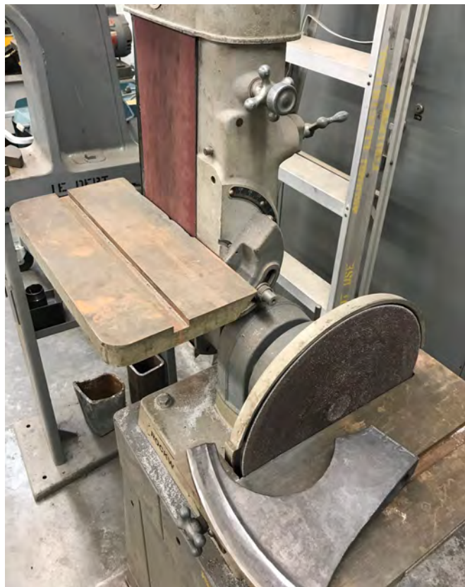
Figure 32: Belt sander used to shave off mill scale
