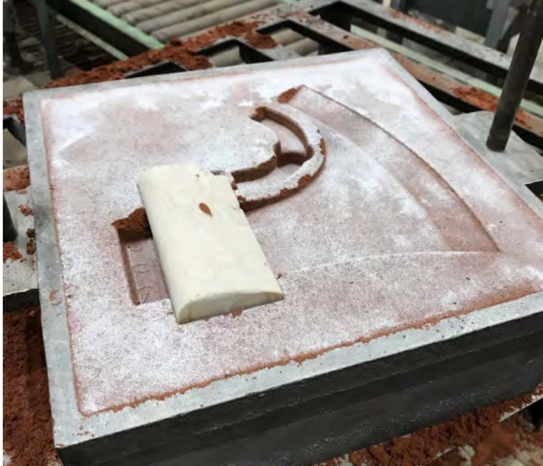
Figure 29: Mold of drag with core box placed inside
