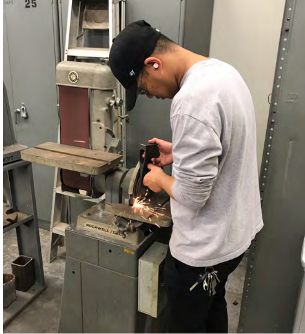
Figure 33: Ben sanding off mill scale on axe head
