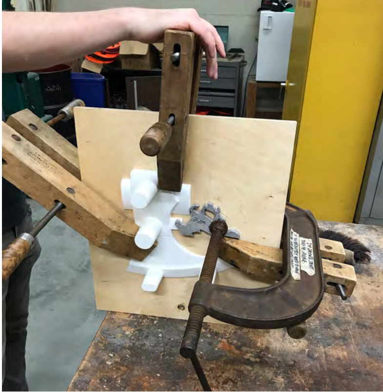
Figure 24: clamping cope and drag patterns for glueing
