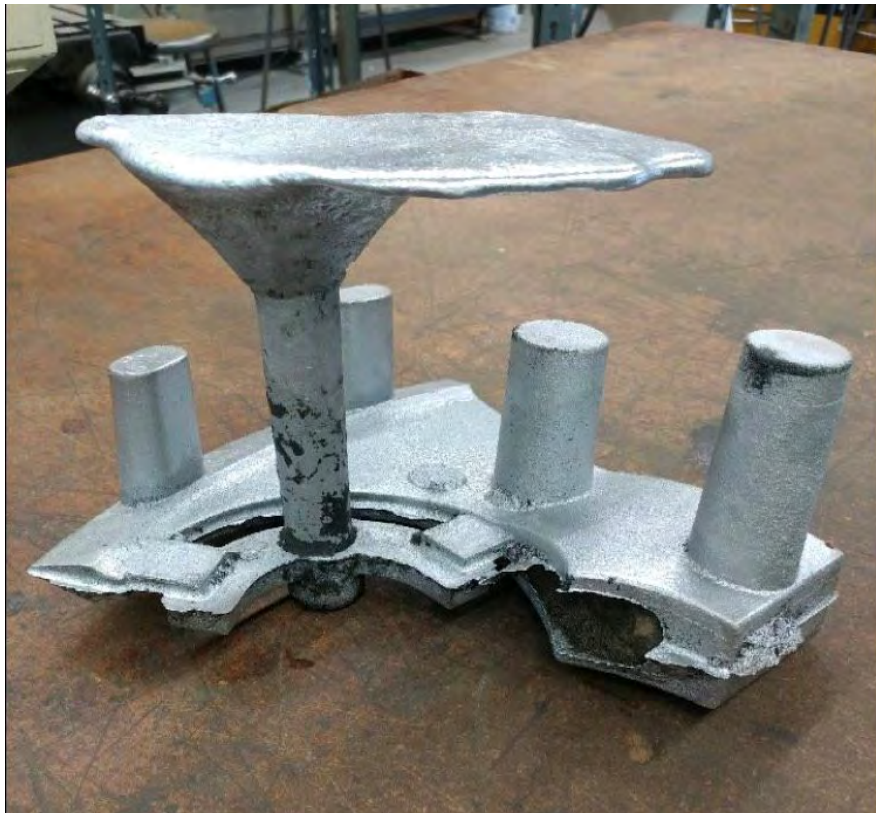
Figure 30: Prototype aluminum casting
