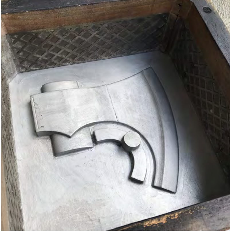
Figure 26: Matchplate with flask on both sides
