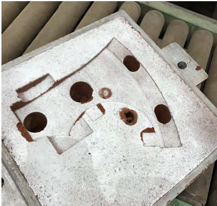
Figure 28: Mold of cope
