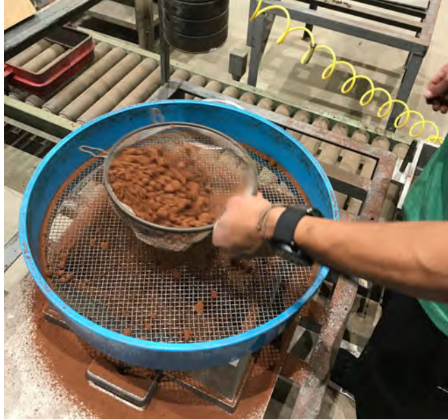
Figure 27: Packing sand with matchplate on bottom
