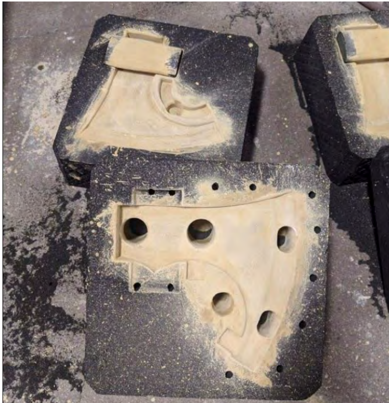
Figure 31: Molds from foundry where steel axes were cast
