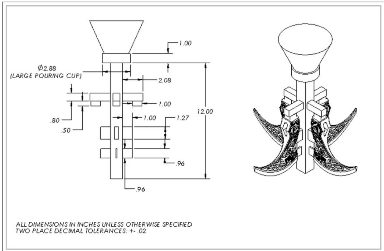
Figure 20: Basic drawing for the most feasible tree pattern design.
