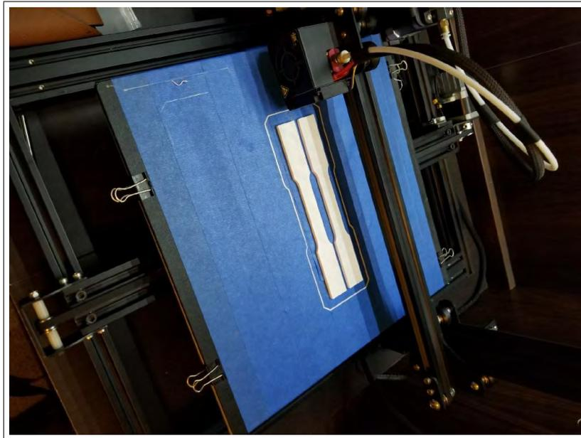
Figure 32: 3D printed Tensile Bars
