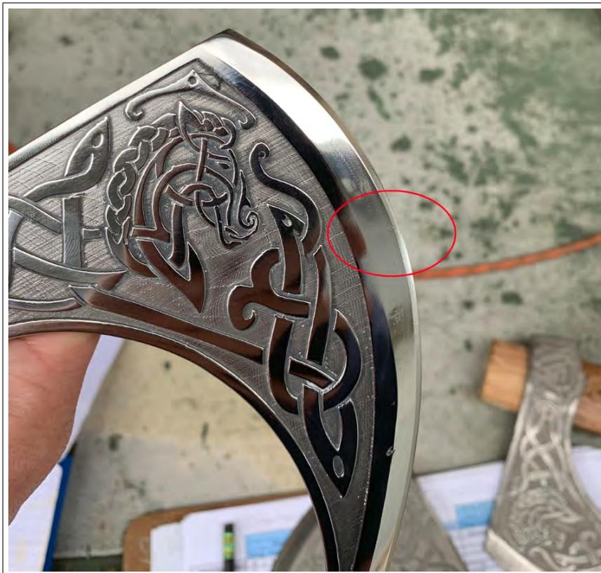
Figure 40: Before Dye Penetrant
