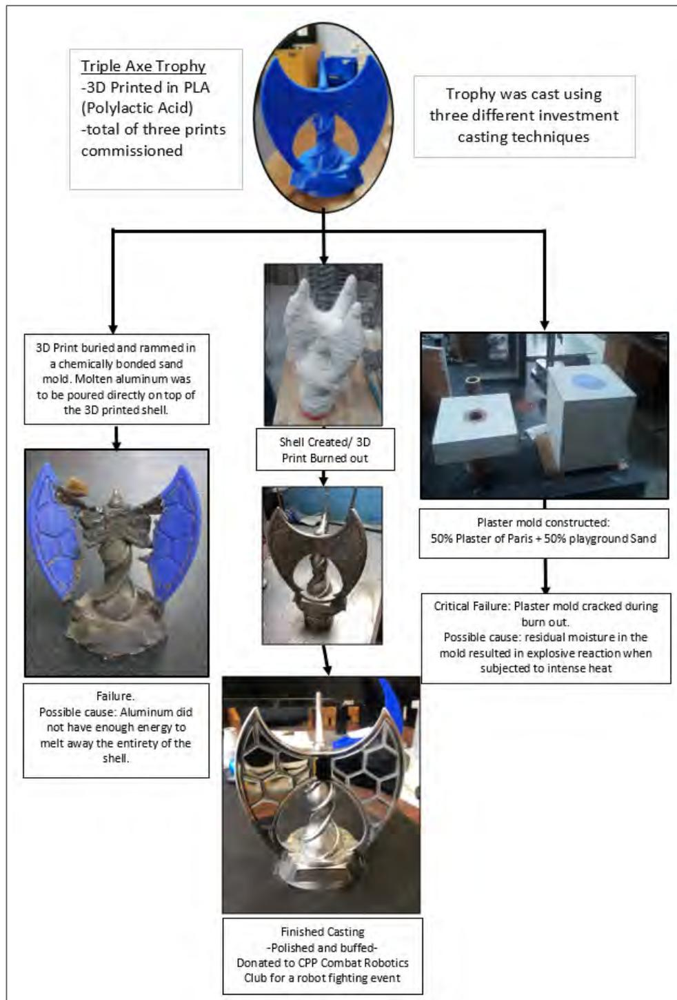
Figure 4: Trophy Process Tree: Three different investment casting techniques (from left to right): lost PLA shell (Evaporative), Traditional investment casting, Plaster of Paris Mold
