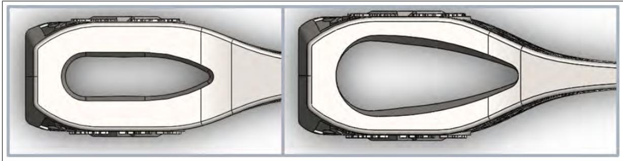
Figure 23: Top view of Axe Head: *Changes in cross sectional thickness and eye dimensions*
