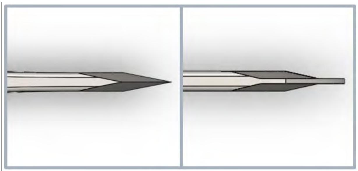
Figure 24: Top view of Axe Blade: *Added flange along the blade edge to be removed in post processing*
