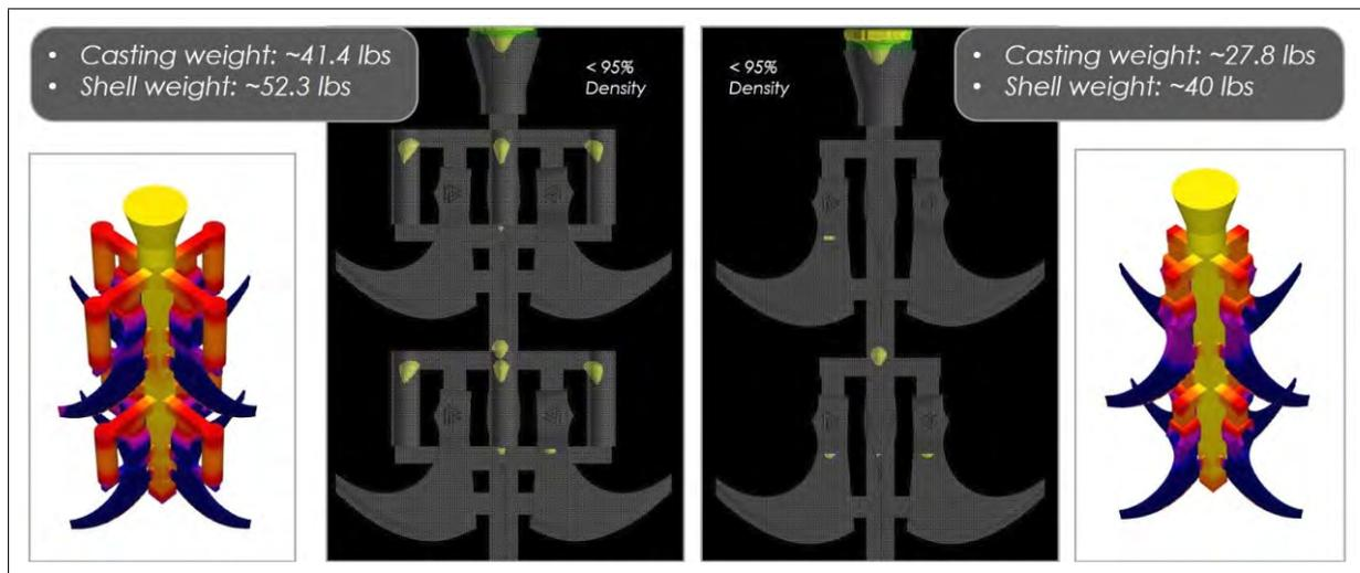
Figure 28: Double Decker Different Running system
