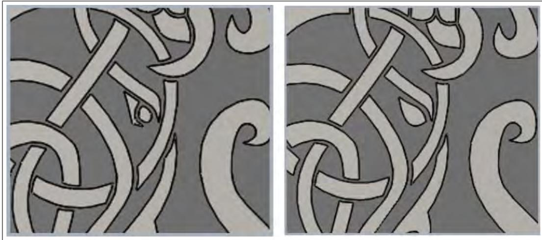
Figure 25: *Some artwork features were found to be too intricate for the 3D printer and needed to be redesigned to prevent misprints.*
