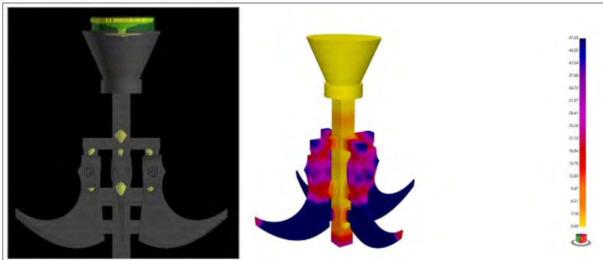
Figure 21: Material Density on the left, Cooling rate on the Right
