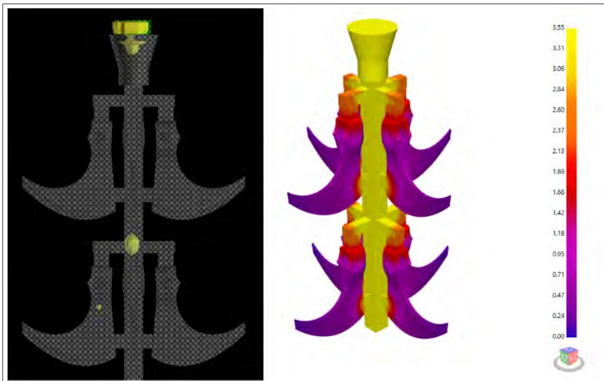
Figure 26: Double Decker tree Assembly: *Material density plot shown to the left, Solidification plot on the right.*
