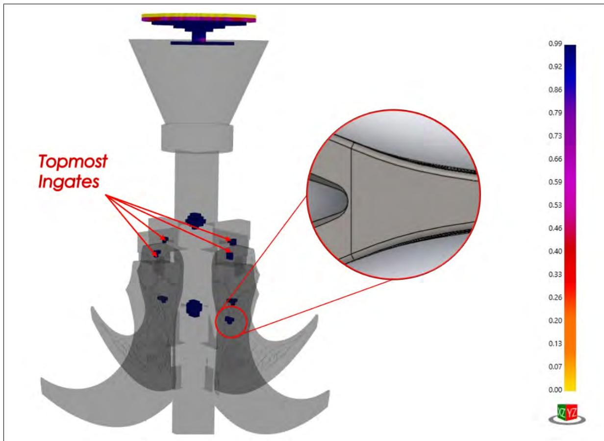
Figure 22: Isometric view of porosity formation
