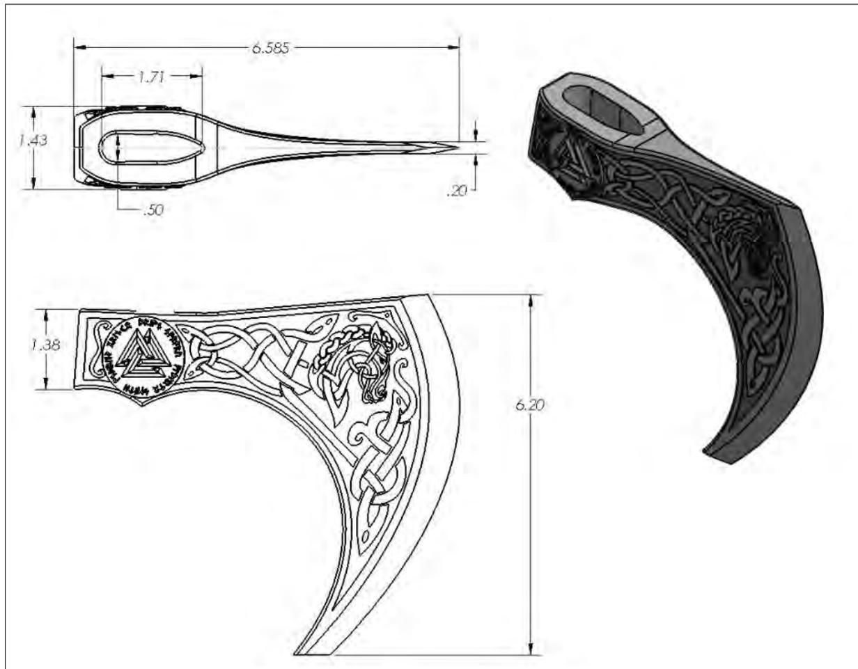
Figure 9: Projected view of axe model with artwork and simple dimensions
