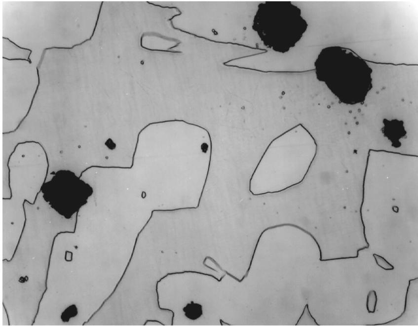
Figure 7. Microstructure of ASTM A890-4A Heat 2 SA, 400X, Oxalic
