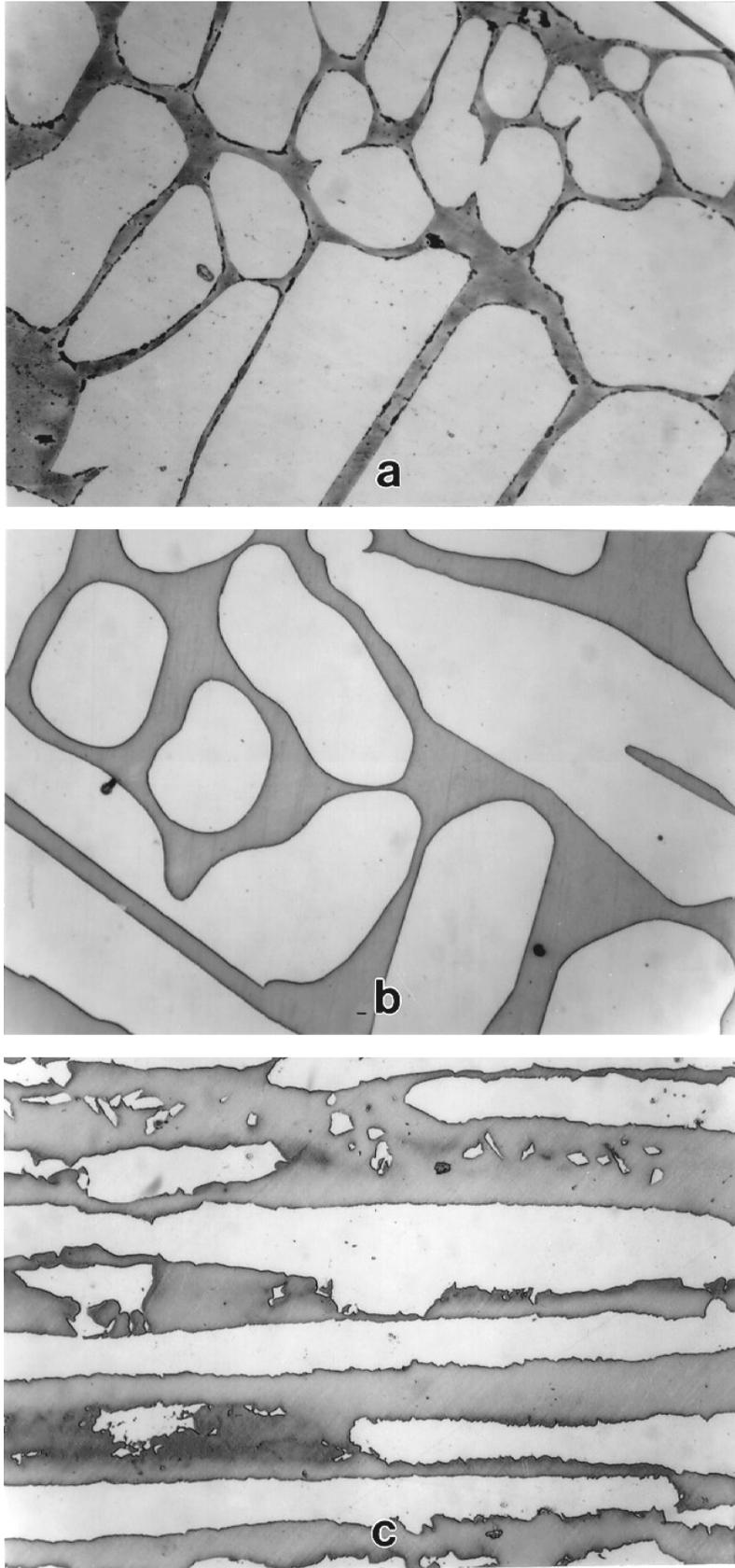
Figure 1-1. Sodium Hydroxide etched structure of ASTM A890-4A (a) As-cast, (b) SA Casting, (c) Wrought Alloy 2205, 400X
