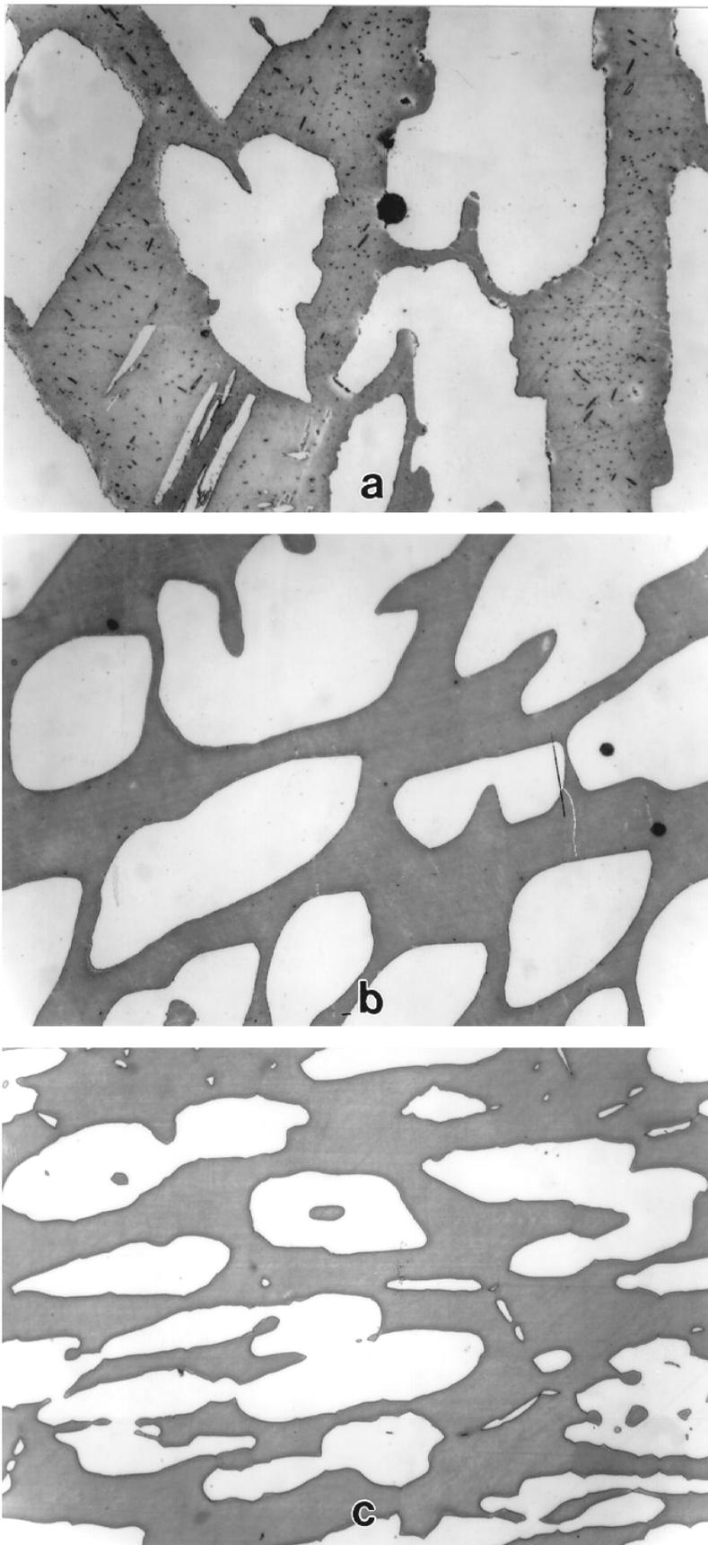
Figure 1-4. Sodium Hydroxide etched structure of ASTM A890-1B (a) As-cast, (b) SA Casting, (c) Ferralium 255, 400X
