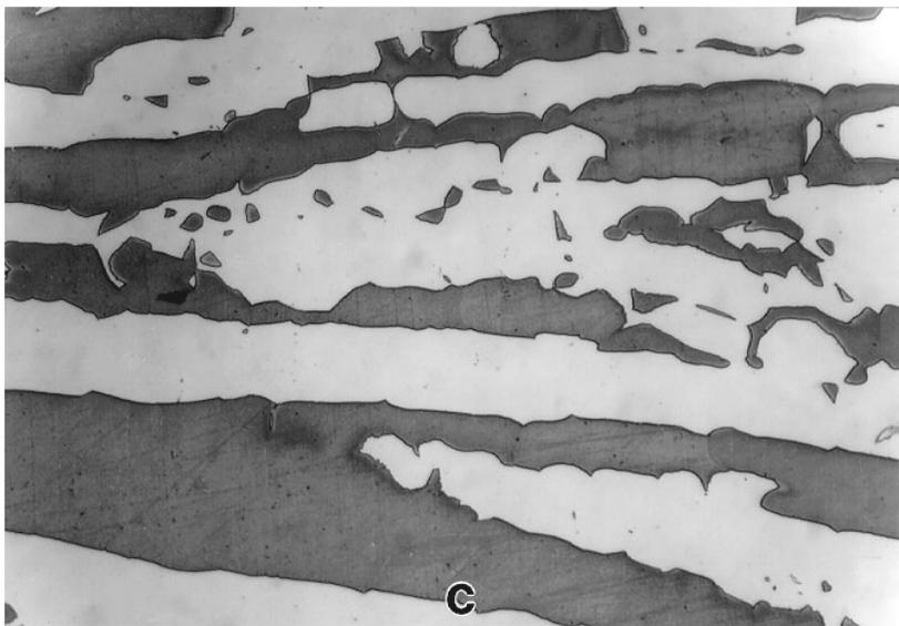
Figure 1-3. Sodium Hydroxide etched structure of ASTM A890-6A (a) As-cast, (b) SA Casting, (c) Zeron 100, 400X
