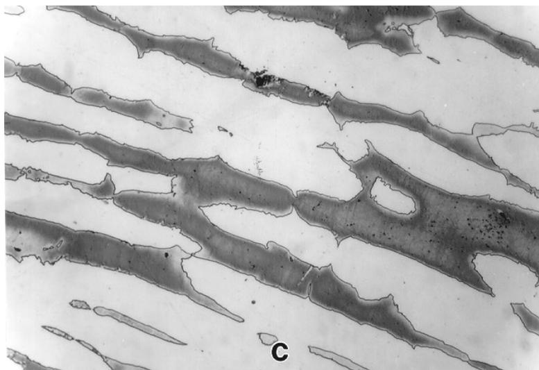
Figure 1-2. Sodium Hydroxide etched structure of ASTM A890-5A (a) As-cast, (b) SA Casting, (c) Wrought Alloy 2507, 400X
